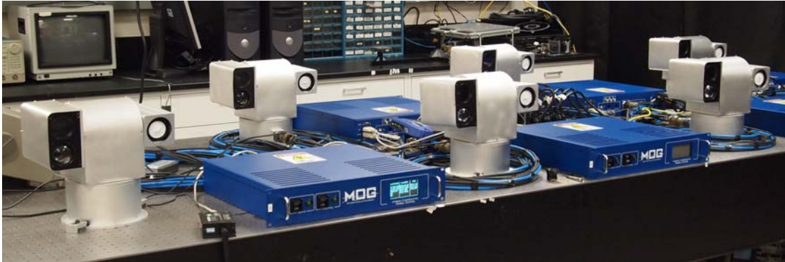
Figure 4.15: Completed FSO/zoom camera pan-tilt platforms.
