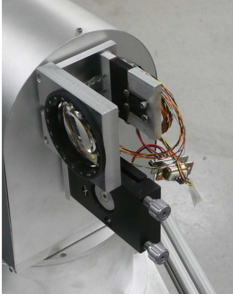
Figure 3.15: Completed beacon assembly. The laser is on bottom in a rotation stage, while the large-area photodiode is mounted above, sitting behind a PCX lens.
