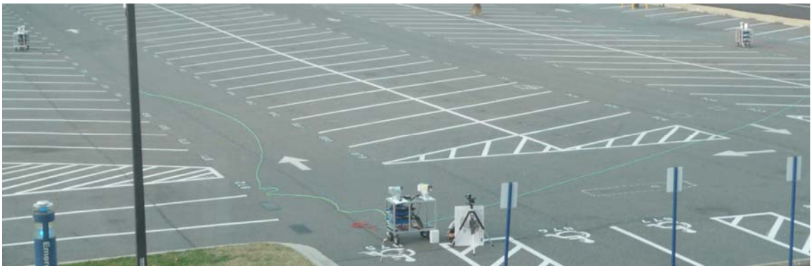
Figure 4.29: Outdoor test-bed. The node in front was the DTCN, sending pointing commands to the other two nodes.
