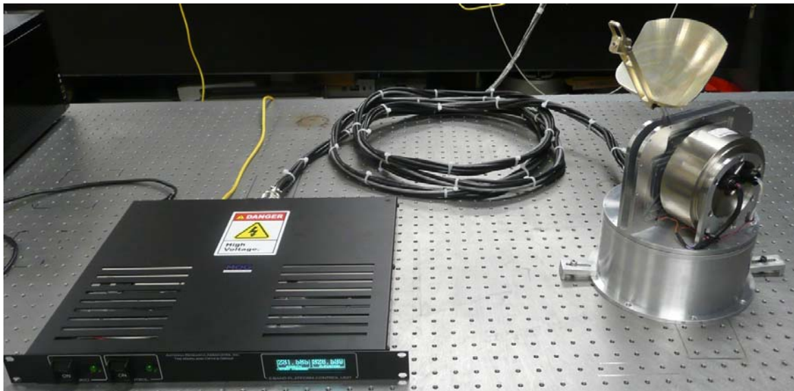
Figure 3.4: E-band platform with antenna and controller
