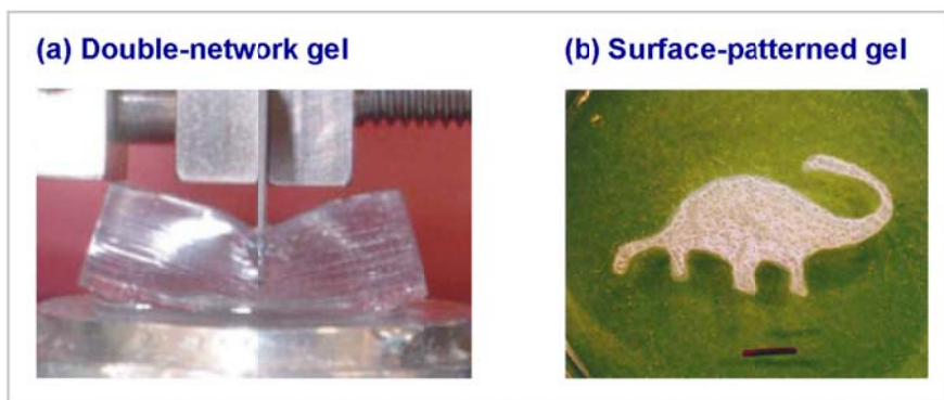
Figure 2.8. Variations of the traditional interpenetrated networks: double-networks 12 and surface-patterned gels. 13
