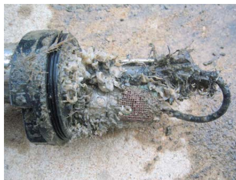
Sensor with the biofouling prevention system after four-week field deployment.
