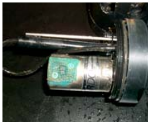
Sensor with the biofouling prevention system after four-week field deployment.
