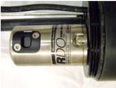
Sensor without the biofouling prevention system after four-week laboratory deployment.
