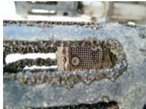
Sensor with the biofouling prevention system after four-week field deployment.
