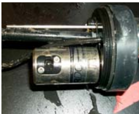
Sensor without the biofouling prevention system after four-week field deployment.
