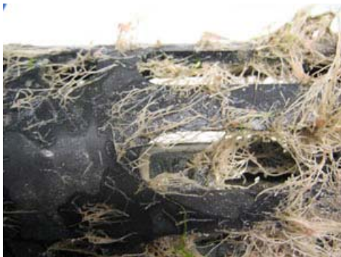
Sensor without the biofouling prevention system after four-week field deployment.
