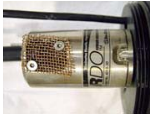
Sensor with the biofouling prevention system after four-week laboratory deployment.
