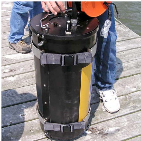
YSI 9600 canister prior to deployment
