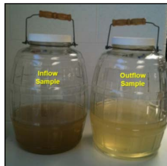
Figure 5. Photograph showing the inflow and outflow composite samples collected during the Feb 29, 2012, rainfall event.
