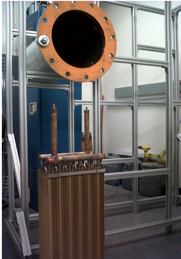
Figure 64: Chiller aluminum frame with one chamber and adsorber
