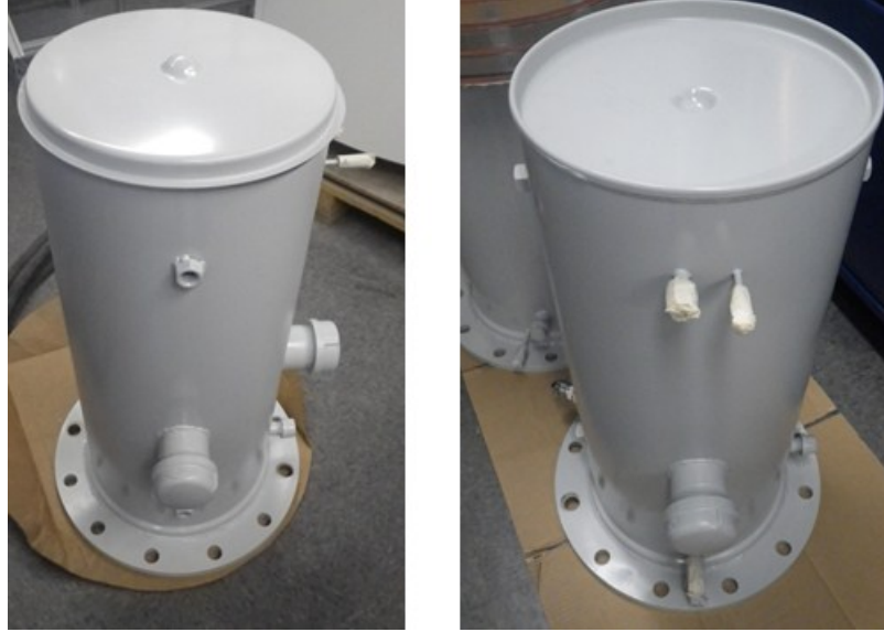
Figure 63: Two vacuum chambers as received from PPI
