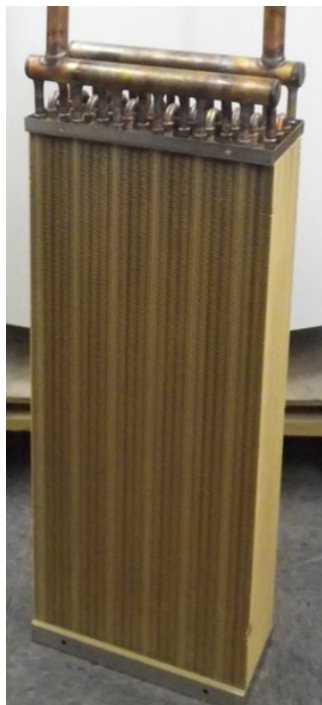
Figure 60: Adsorber heat exchanger used in prototype chiller
