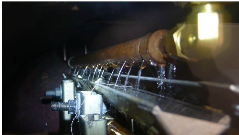
Figure 69: Falling film distributor in operation, zoomed out
