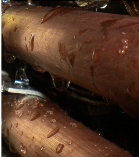
Figure 70: Initial wettability of sanded and solvent-cleaned copper tubes
