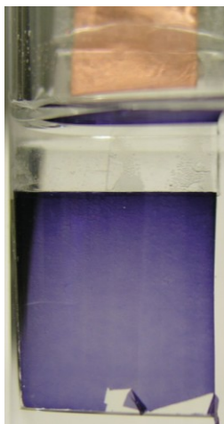
Figure 3.2 ITO 1.26 cm 2 with copper and tape after polymerization of PMProDot.
