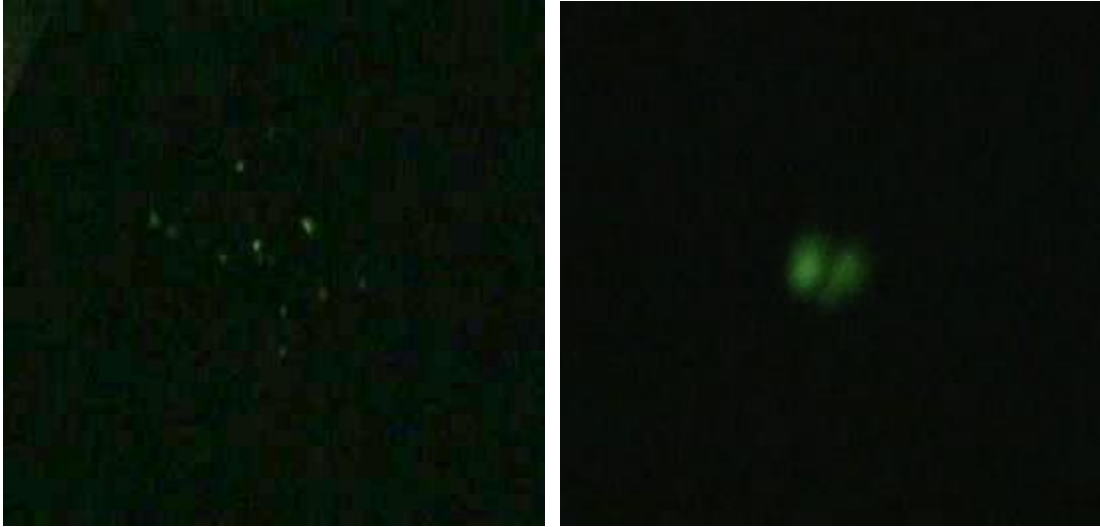
Figure 3.12: (left) Field Ion Image of a Pd/W tip, Imaging at 4.8 kV, He pressure 3 \times 10^{-5} Torr. (right) Field Emission Image.
