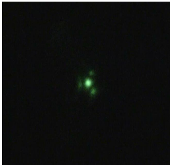
Figure 3.11: FIM image after exposure to air, imaging voltage 1.9 kV.
