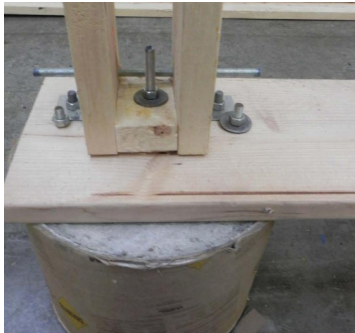
Figure 91 Full scale model of foundation, base plate, and column.
