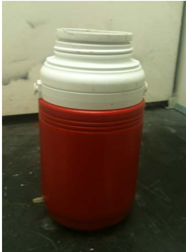
Figure 2-3. An insulated plastic dewar that has the tube (2 mm inside diameter and 120 mm of length)
