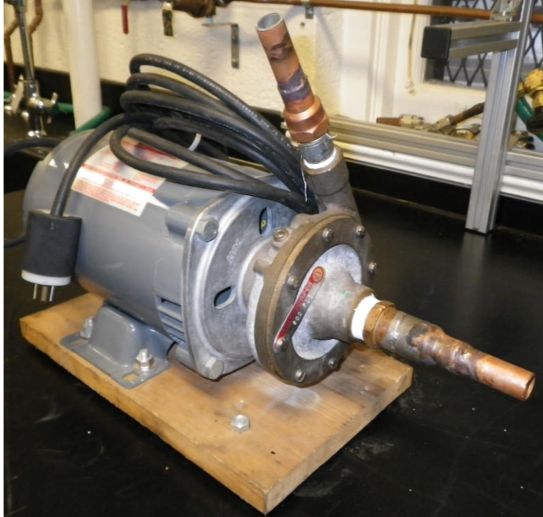
Figure 14: Water Pump for Wetting Water Loop
