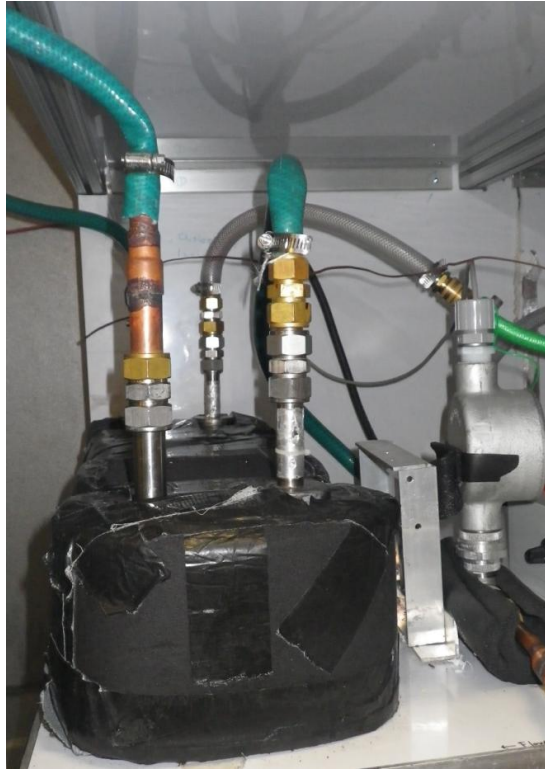
Figure 32: Wetting Water Side Plate HX
