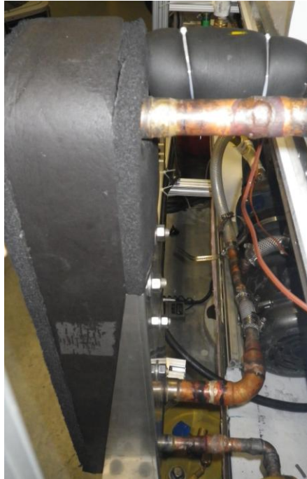
Figure 34: The Hot Water Loop Plate HX
