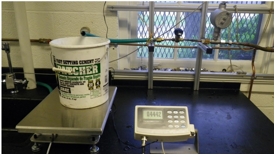
Figure 48: Water Flow Meter Calibration Set-up
