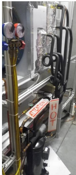
Figure 35: Secondary Refrigerant Loop
