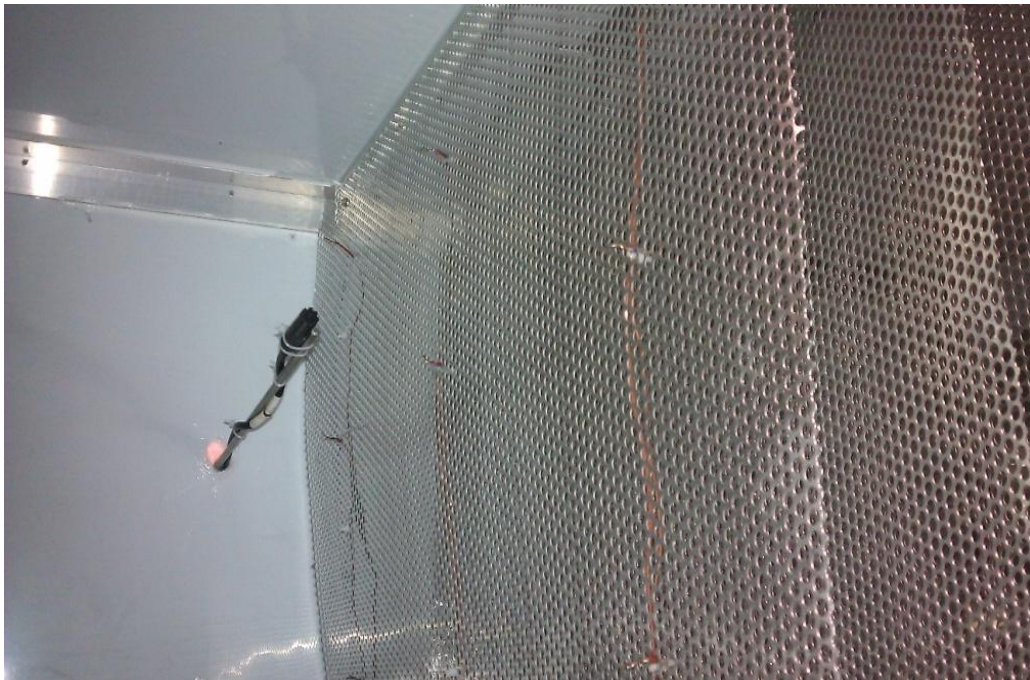
Figure 29: RH Sensor, TC Grid and Air Flow Settling Means
