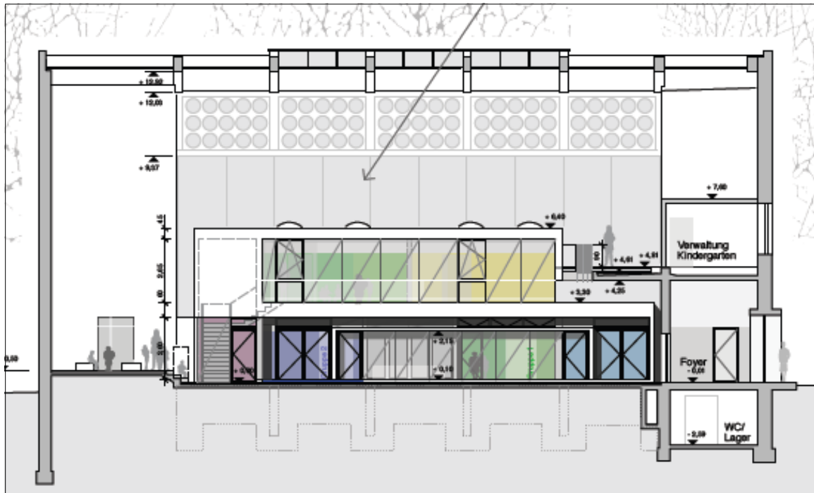
Figure 24: Longitudinal section of the Bethlehemkirche with the kindergarten insertion (Courtesy of Stölken Schmidt Architekten)
