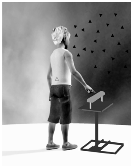
Figure 4.1. Experimental set-up in which a child is performing the multi-sensory posture task (room illumination not dimmed for illustrative purposes; fewer dots are plotted for a clear view of child's posture).
