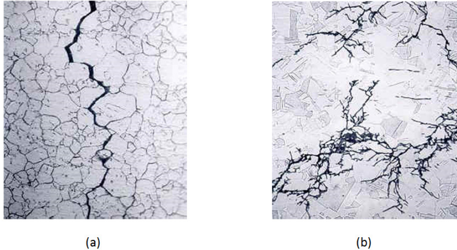
Figure 2.1 - (a) Intergranular crack: Caustic SCC in the HAZ of Type 316L Stainless Steel NaOH reactor vessel (b) Transgranular Crack: SCC in 308 Stainless Steel Weld in Aqueous Chloride at 95C [8]
