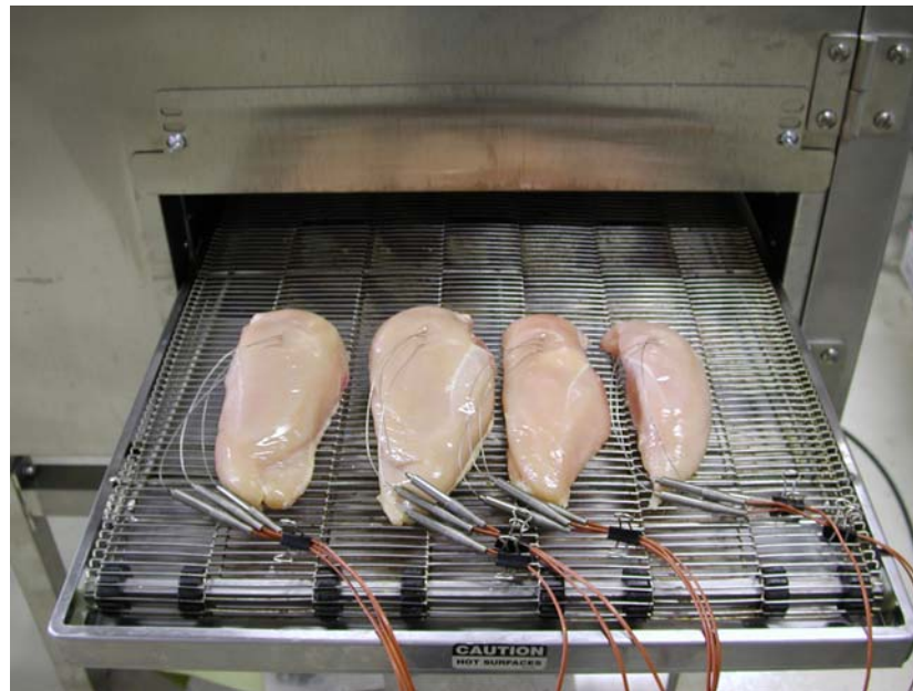
Figure 16. Four chicken breasts before cooking with three TCs inserted into the thickest part of each one.
