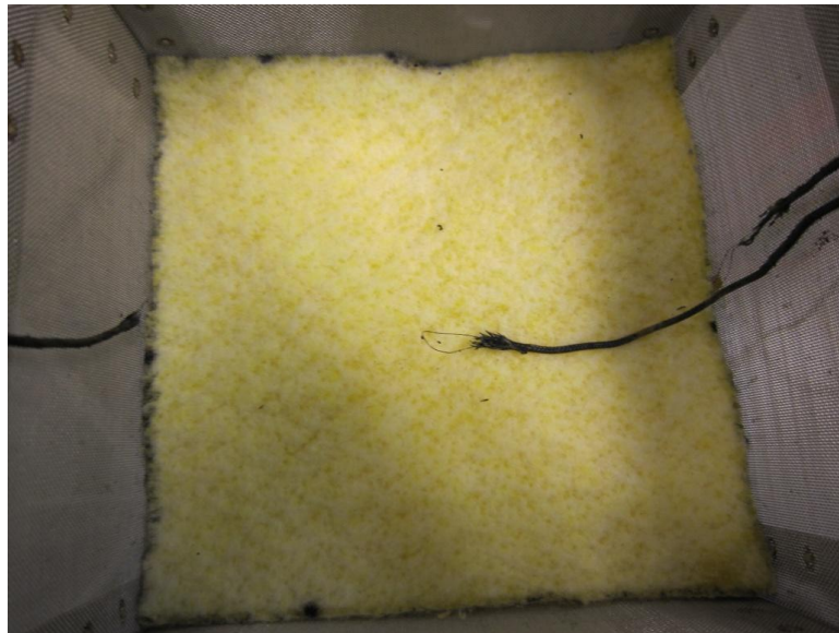
Figure 3.16: Thermocouple Placement In the Center and On the Surface of the Sample
