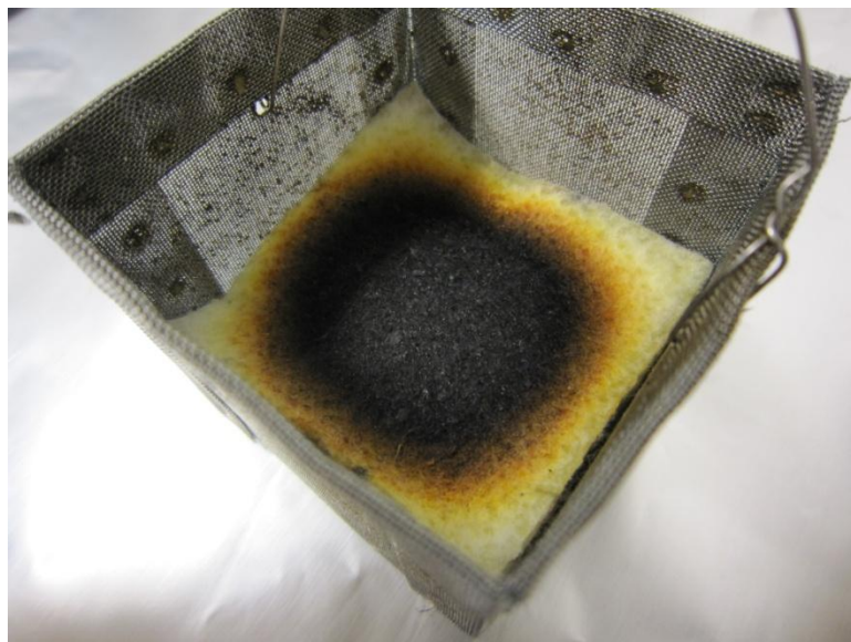
Figure 4.2: Charred Center of a Sample
