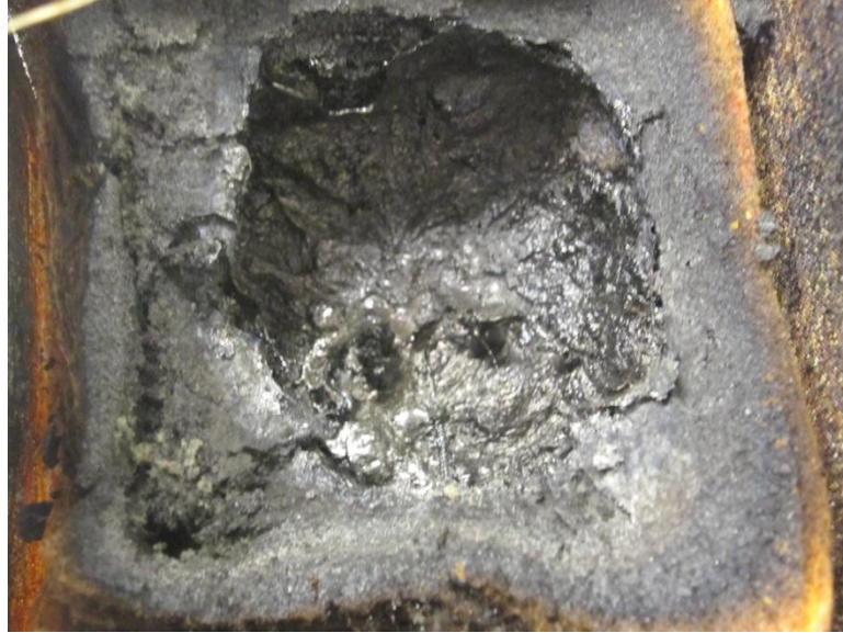
Figure 4.5: A Very large Void Created Around the Center Thermocouple
