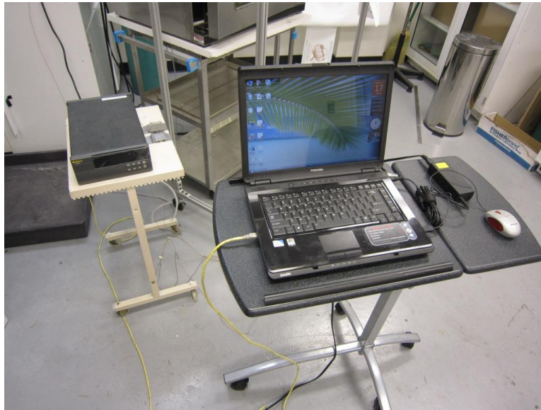
Figure 3.7: Fluke 2645A NetDAQ System Connected to the Computer
