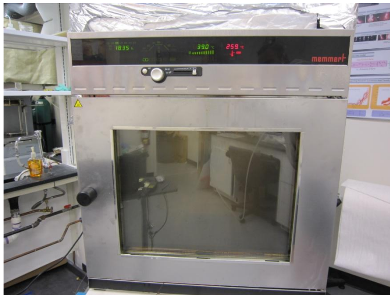
Figure 3.1: The Memmert UFE500 Forced Controlled Convection Oven
