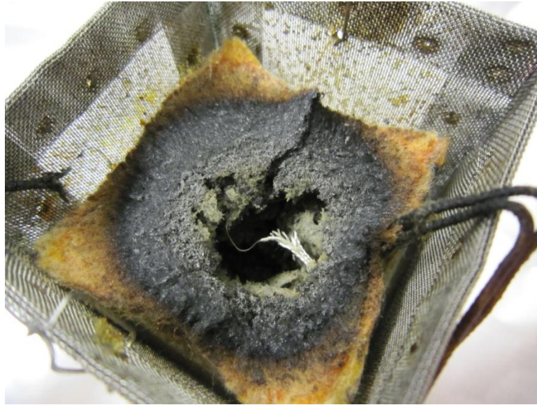
Figure 4.3: A Void Created Around the Center Thermocouple
