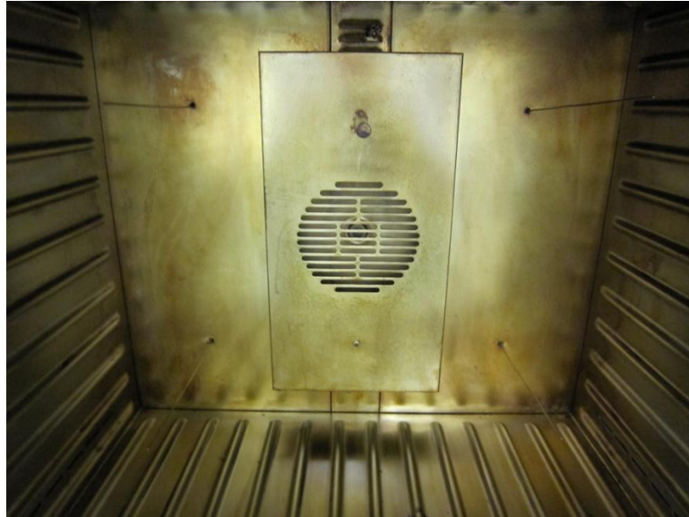
Figure 3.2: Inside of Oven Showing Thermocouple Placement
