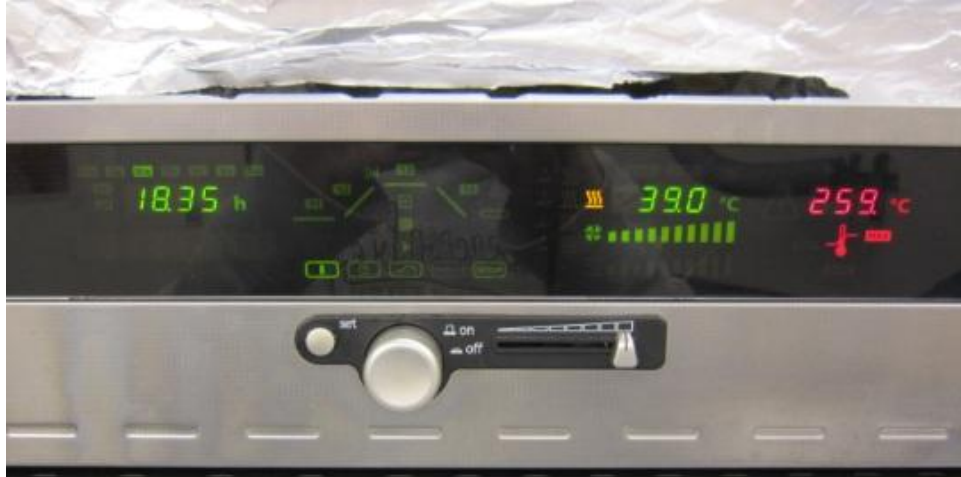
Figure 3.3: Front Display of Oven with On/Off Switch and Adjustment Dial
