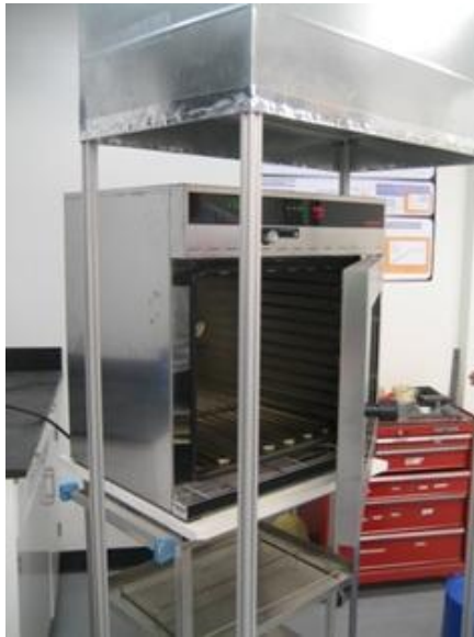
Figure 3.10: Portable Hood Positioned Over the Open Oven Door
