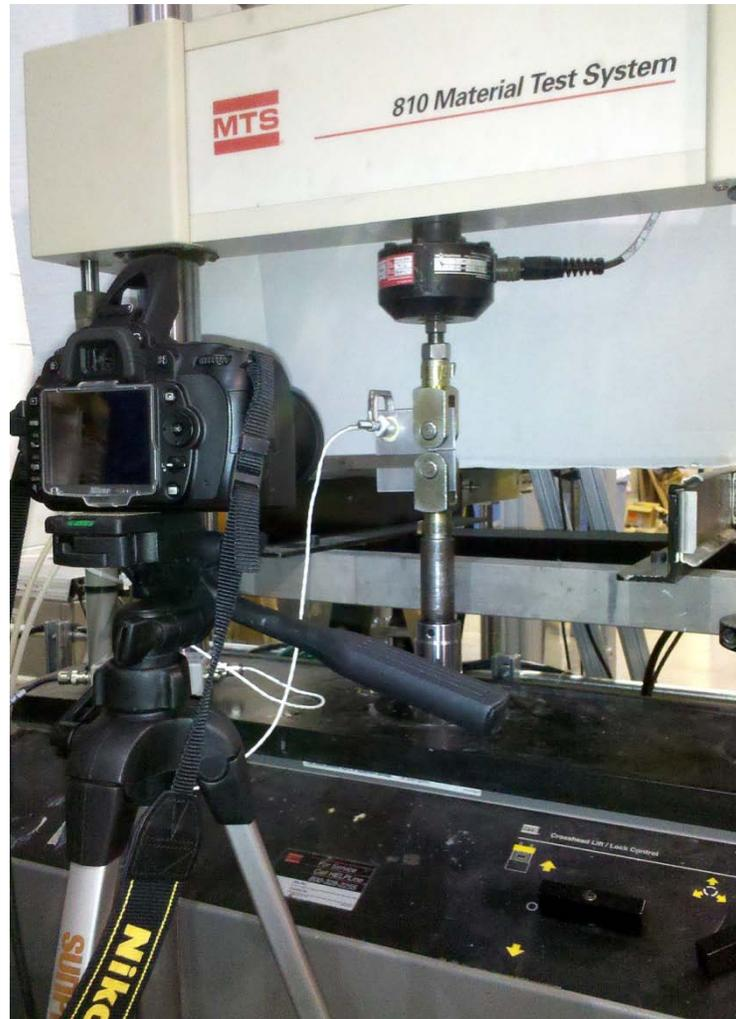
Figure 2.8 – Test setup for crack measurement using digital photography.
