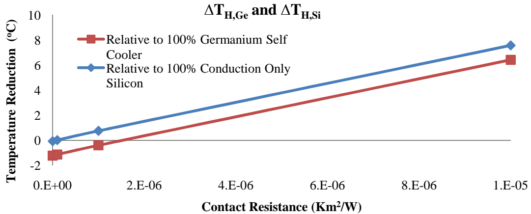
Figure 126: Bi-Layer Self Cooler, Temperature Reduction as a function of Contact Resistance for 1400μm Cooler size, 85% Germanium, and 500μm die thickness case
