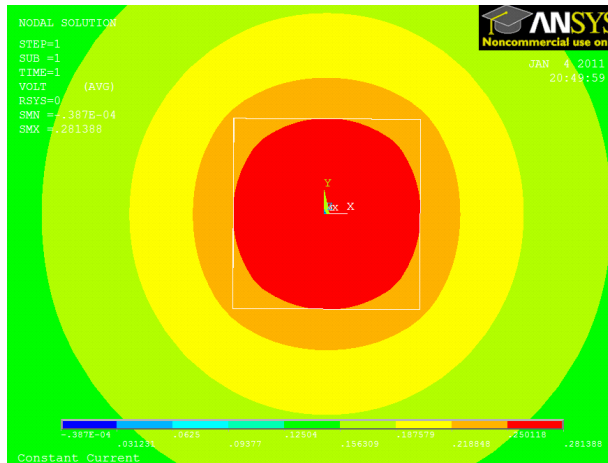
Figure 57: Hotspot off, Constant Current Self Cooler, Electric Potential Plot, 100 \mu m die 630 \mu m wide Cooler and 1.06A
