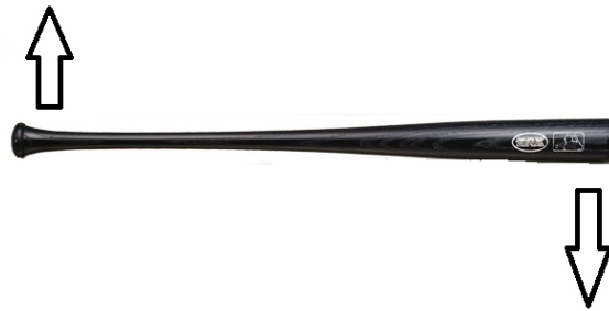
2nd mode has only one node in the center, so the bat experiences only rotational translation.
