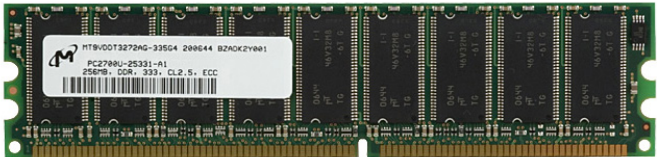
Figure 3.7: DDR333 SDRAM DIMM, 256MB with ECC
