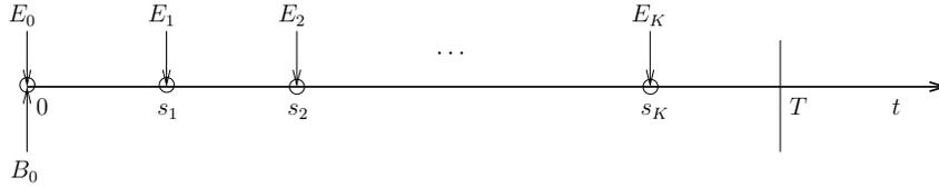
Figure 5.3: System model with all bits available at the beginning. Energies arrive at points denoted by  $\circ$ .
