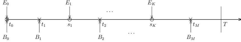
Figure 5.2: System model with random packet and energy arrivals. Data packets arrive at points denoted by  $\times$  and energies arrive (are harvested) at points denoted by  $\circ$ .
