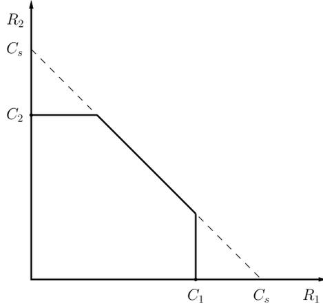
Figure 3.1: The capacity region for a two-user multiple access system.
