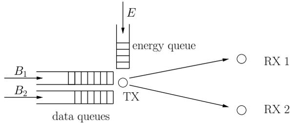
Figure 6.1: An energy harvesting two-user broadcast channel.
