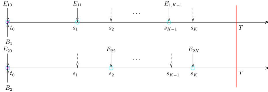
Figure 7.2: System model with all packets available at the beginning. Energies arrive at points denoted by  $\circ$ .
