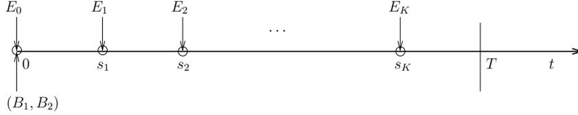
Figure 6.2: System model.  $(B_1, B_2)$  bits to be transmitted to users are available at the transmitter at the beginning. Energies arrive (are harvested) at points denoted by  $\circ$ .  $T$  denotes the transmission completion time by which all of the bits are delivered to their respective destinations.
