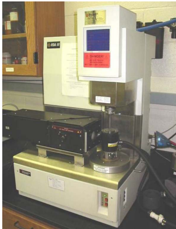
Figure 2.9. Photograph of the Rheometer RDA-III strain-controlled rheometer being operated in a cone-and-plate geometry.
