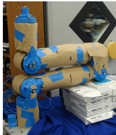
Figure 4.4 Ranger with reflective surfaces covered and markers attached in preparation for Vicon testing.
