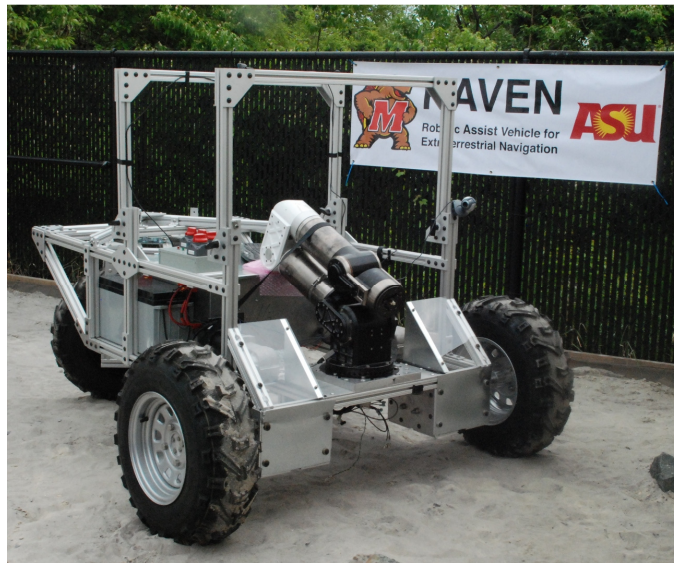
Figure 5.1 The RAVEN astronaut assistance rover. In this image, a nonfunctional Ranger manipulator occupies the location in the front of the vehicle where Ranger Mark I will be mounted. From [30].
