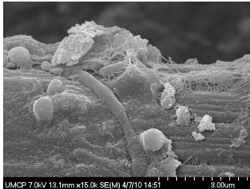
Figure 4-23. Micrograph of anodic fiber taken from the bottom half of Reactor B. Example of a filamentous bacterium surrounded by cocci.
