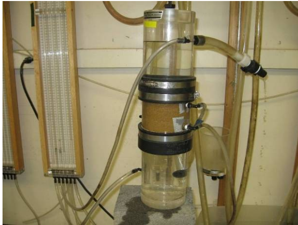
Figure 3-2. Gradient Ratio Test with Constant Head Permeameter
