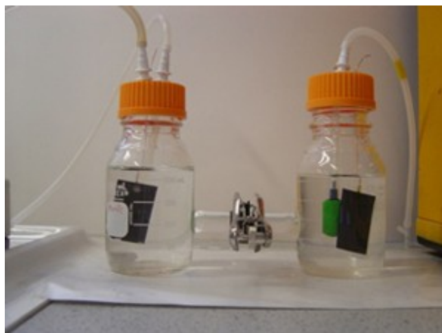
Figure 2-2. Two-chambered H-type MFC in which the cathode chamber is aerated and a cation-specific membrane separates the anode from the cathode (from: www.engr.psu.edu/ce/ENVE/logan )
