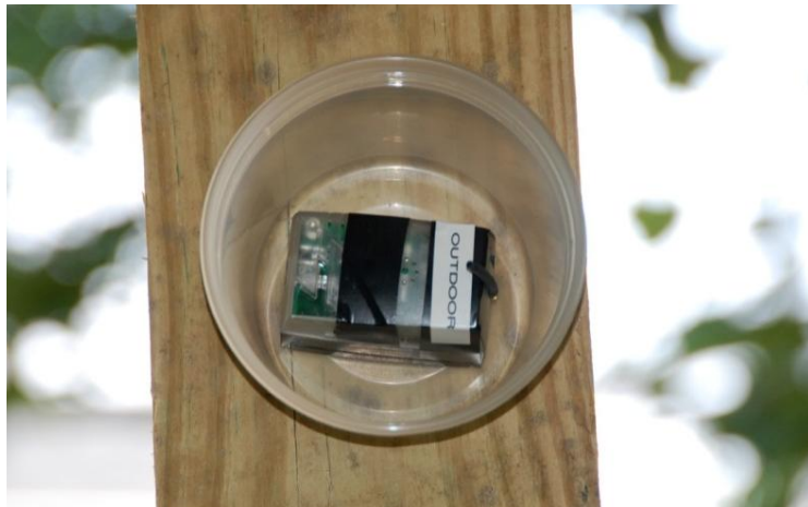
Figure 3.9 Photograph of the Outdoor Mote in Plastic Housing (without the cover)
