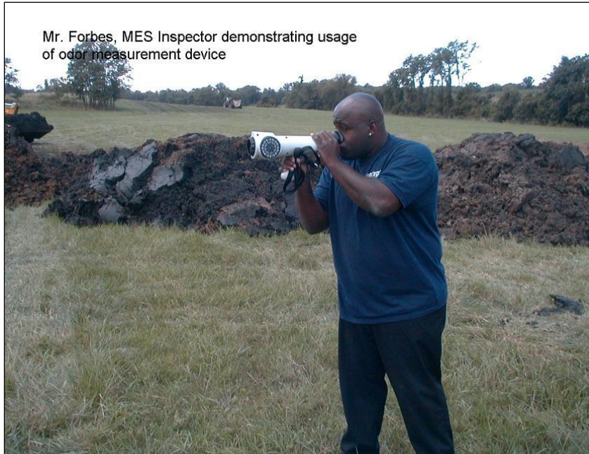
Figure 3.4: MES Inspector with Nasal Field Olfactometer
