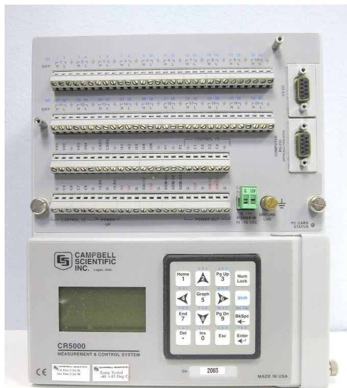
Figure 12 - Campbell Science CR5000 Data Logger
