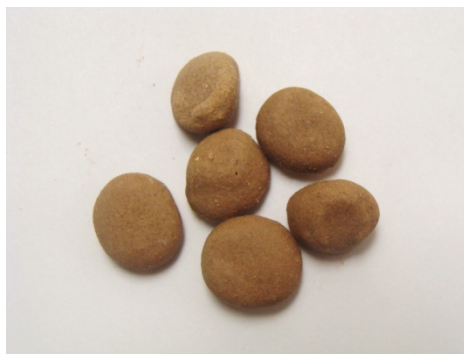
Figure 5.6c: Biomeal pellets created using 20% sodium citrate and 10% calcium chloride
