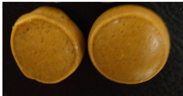
Figure 5.7a: Biomeal-alginate gels formulated using 1.5% sodium alginate and 10% calcium chloride
