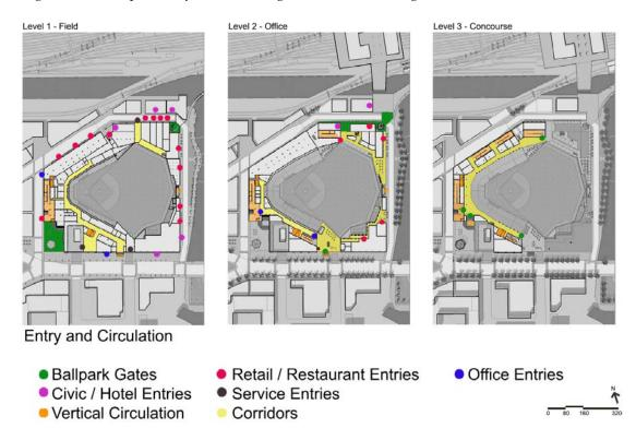
Fig. 8-26 – Ballpark Entry and Circulation Diagram
