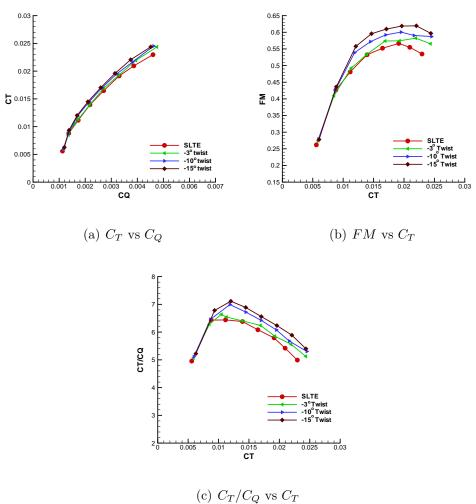
Figure 4.32: Performance comparison for various blade twists for micro-scale single rotor, SLTE geometry.
