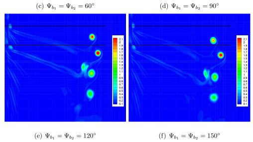
Figure 5.19: Vorticity magnitude contours in a fixed plane in space for full-scale coaxial system at different instances in time for full-scale coaxial system (case 7).
