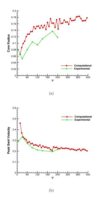
Figure 4.29: Tip vortex viscous core radius (a) and Peak tip vortex swirl velocity (b) comparison with experimental data [29] with wake age for micro-scale single rotor.
