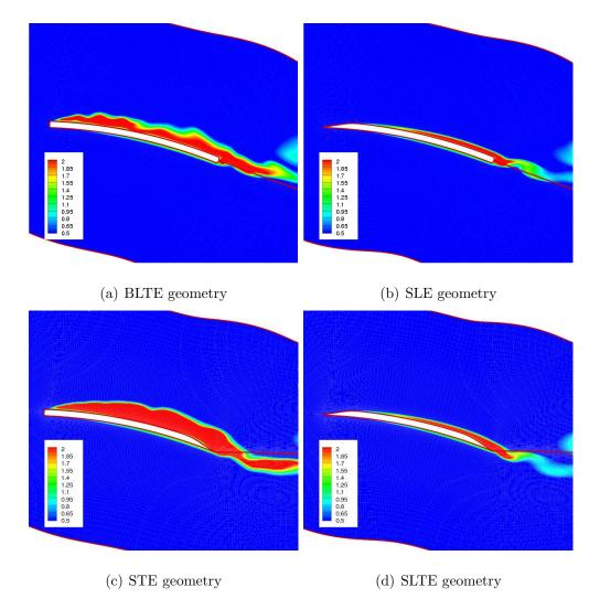
Figure 4.17: Eddy Viscosity contours at 0.95R for micro-scale single rotor,  $12^\circ$  collective setting.
