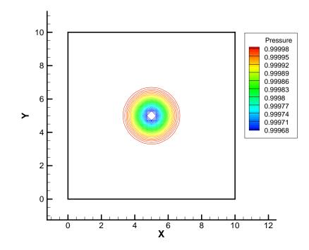
Figure 3.1: Computational domain and initial pressure contours for isentropic vortex convection.
