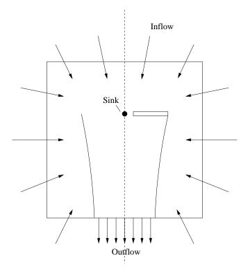
Figure 2.9: Schematic of point-sink boundary condition.
