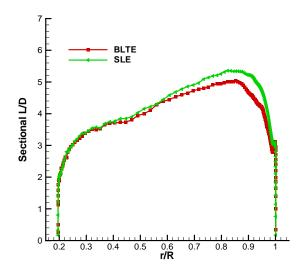
Figure 4.8: Sectional L/D distributions for BLTE and SLE geometry of microscale single rotor, 12° collective setting.
