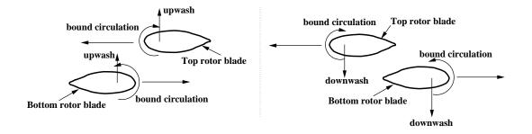
Figure 5.5: Schematic of the loading effect in coaxial system.
