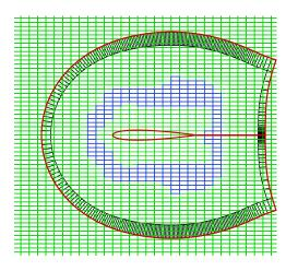
Figure 3.15: Connectivity obtained by manually removing fringe points from baseline IHC methodology. blue: fringe points of background mesh; black: fringe points of airfoil mesh; green: field points of background mesh.
