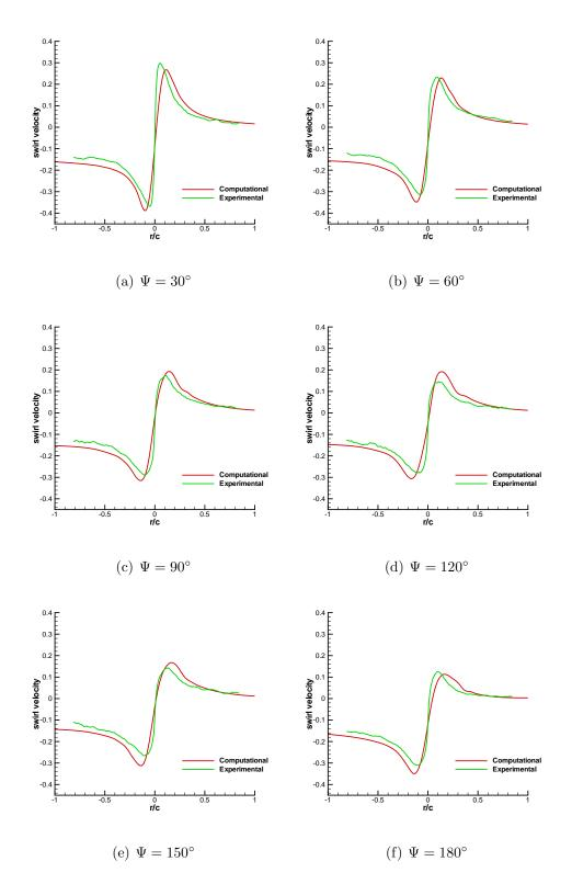
Figure 4.27: Vortex swirl velocity profile (non-dimensionalized by tip speed) comparison between computational BLTE geometry and experimental baseline geometry [29] for micro-scale single rotor, 12° collective setting.
