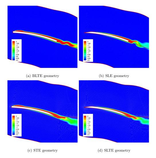
Figure 4.16: Eddy Viscosity contours at 0.8R for micro-scale single rotor,  $12^\circ$  collective setting.
