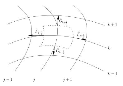
Figure 2.6: Schematic showing computational cell.
