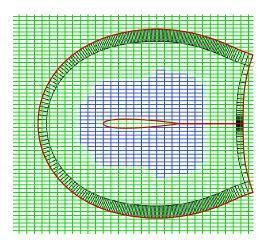
Figure 3.13: Connectivity using baseline implicit hole-cutting methodology. blue: fringe points of background mesh; black: fringe points of airfoil mesh; green: field points of background mesh.
