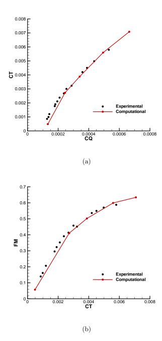
Figure 3.22: Performance comparison for Harrington single rotor-2 [49] with old hole-cutting method and old blanking technique.
