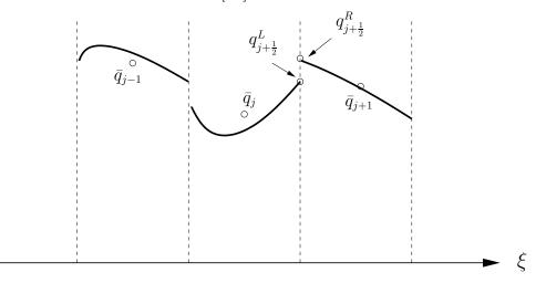
Figure 2.7: Schematic of one dimensional piecewise reconstruction.
