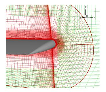
Figure 2.5: Sample overset grid in a hovering rotor simulation. Red: Blade mesh, Green: Background mesh.
