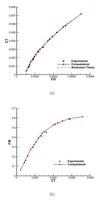
Figure 3.21: Performance comparison for Harrington single rotor-2 [49].
