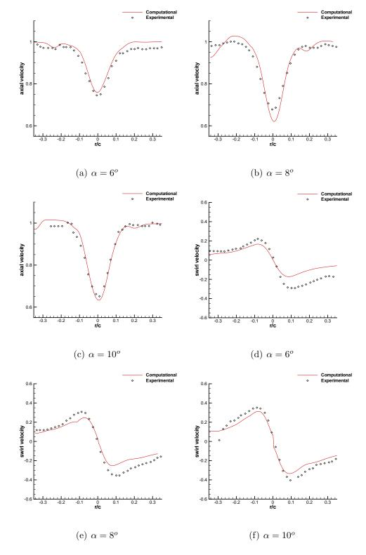
Figure 3.9: Swirl and axial velocity profile with experimental data [86] at x/c = 4, Re = 9040.
