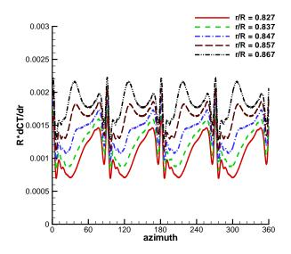
Figure 5.11: Temporal variation in sectional thrust  $\left(R\frac{dC_T}{dr}\right)$  at selected spanwise locations for the bottom rotor of full-scale coaxial system (case 3).
