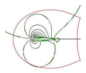
Figure 3.14: Comparison of pressure contours for single mesh and two mesh system using baseline implicit hole-cutting. black: single mesh system; red line: airfoil mesh, green line: background mesh.
