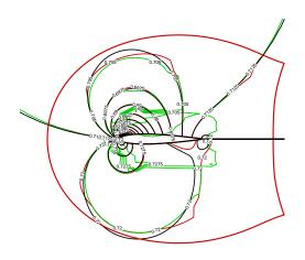
Figure 3.16: Comparison of pressure contours for single mesh and two mesh system using smaller fringe layer thickness and no *iblank* array. black line: single mesh; red line: airfoil mesh, green line: background mesh.
