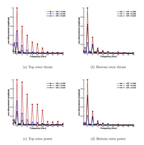
Figure 6.5: Effect of rotor spacing on the frequency distribution, normalized by the amplitude of 4/rev frequency of the h/R = 0.268 case, for micro-scale coaxial system.
