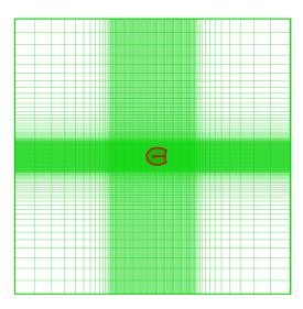
(b) Two mesh system (267  $\times\,65$  airfoil mesh and  $151 \times 151$  background mesh
