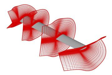
Figure 2.2: Near body C-O mesh at the blade root and tip.
