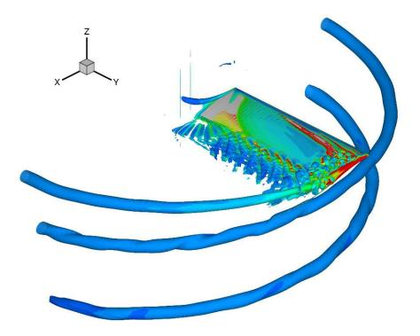
Figure 4.23: Iso-surfaces of second invariant of velocity magnitude (colored by vorticity magnitude), q = 1.0, at  $12^{\circ}$  collective setting for micro-scale single rotor, BLTE geometry.
