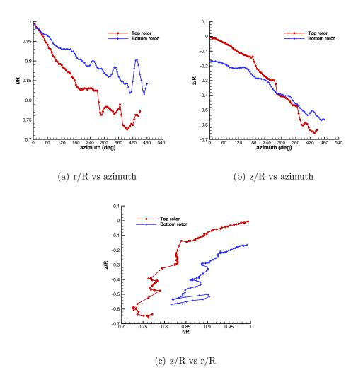
Figure 5.18: Wake trajectory for full-scale coaxial system (case 7) when the blades are aligned.
