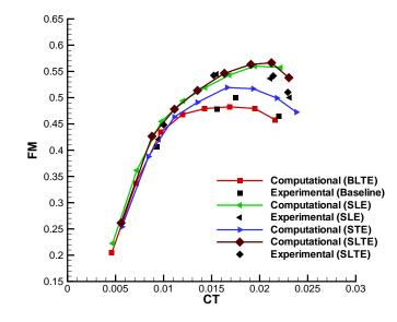
Figure 4.5: Performance comparison  $(FM \text{ vs } C_T)$  with experimental data [29] for micro-scale single rotor.
