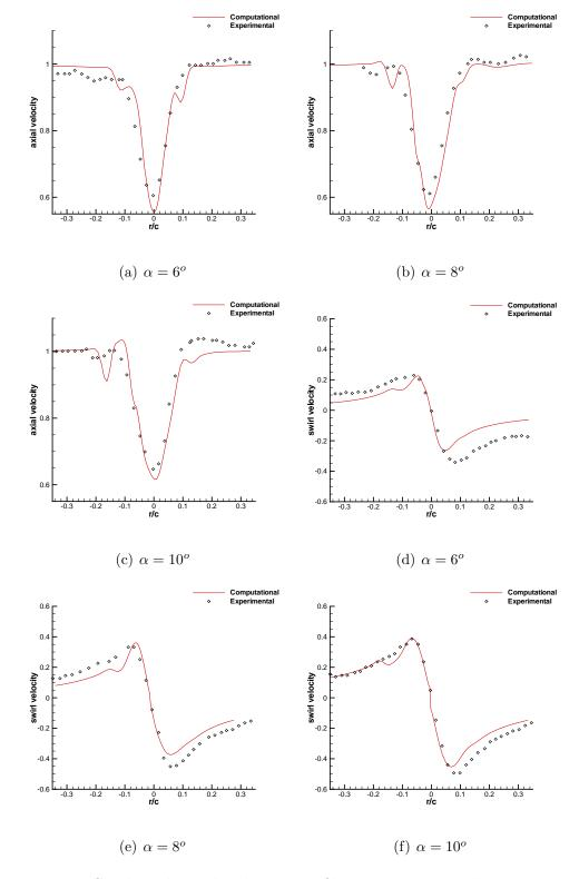
Figure 3.8: Swirl and axial velocity profile comparison with experimental data [86] at x/c = 1, Re = 9040.
