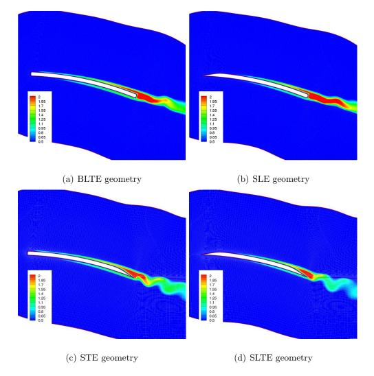
Figure 4.15: Eddy Viscosity contours at 0.6R for micro-scale single rotor,  $12^\circ$  collective setting.
