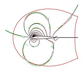
Figure 3.18: Comparison of pressure contours for single mesh and two mesh system using smaller fringe layer thickness and iblank = 1 for fringe points. black line: single mesh; red line: airfoil mesh, green line: background mesh.
