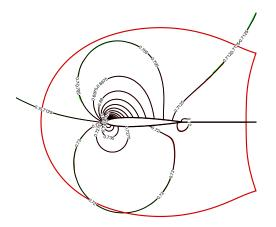
Figure 3.19: Comparison of pressure contours for single mesh and two mesh system using smaller fringe layer thickness and iblank = -1 for fringe points. black line: single mesh; red line: airfoil mesh, green line: background mesh.
