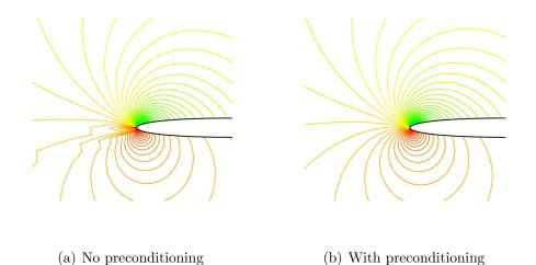
Figure 3.5: Pressure contours for flow over NACA 0006 airfoil at M = 0.05.
