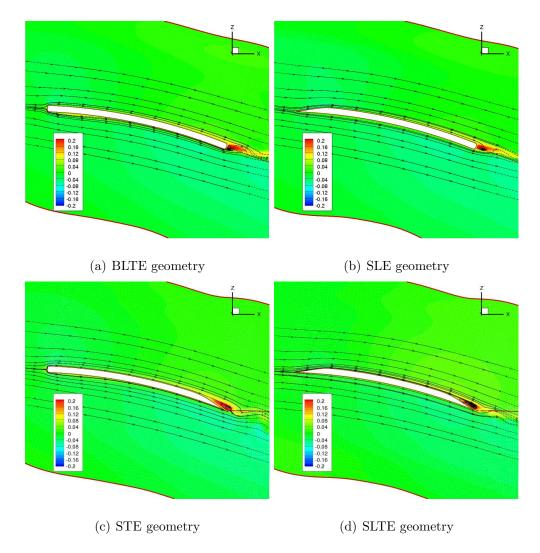
Figure 4.18: Radial Velocity contours along with streamlines at 0.4R for microscale single rotor,  $12^{\circ}$  collective setting.
