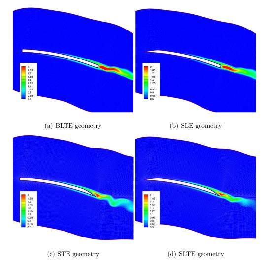
Figure 4.14: Eddy Viscosity contours at 0.4R for micro-scale single rotor,  $12^{\circ}$  collective setting.
