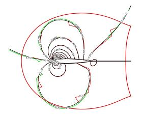
Figure 3.17: Comparison of pressure contours for single mesh and two mesh system using smaller fringe layer thickness and iblank = 0 for fringe points. black line: single mesh; red line: airfoil mesh, green line: background mesh.
