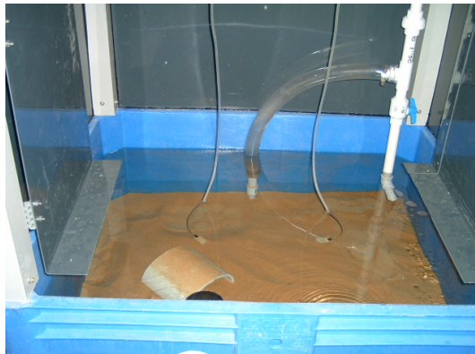
Figure 2.2. Experimental tank system with individually enclosed tanks. (A) The blue tanks on the bottom are the DB system while white tanks on the top are the DT system. (B) Each tank was enclosed with black plastic PVC sheeting (0.32 cm thick) to create a light tight environment.
