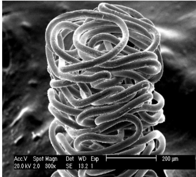
Figure 24. SEM SE (20KV, 300x) image of a Cinch CIN::APSE contact
