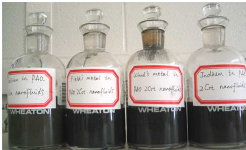
Figure 3-3 As-prepared nanofluids by using the nanoemulsification method at room temperature. From left to right are: gallium, Field's Metal, Wood's metal and indium nanoparticles in PAO nanofluids
