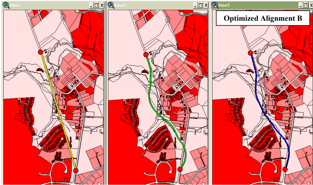
(a1) Optimized Alignment with C_T = C_L + C_S + C_M (Case1) (a2) Optimized Alignment with C_T = C_L + C_S + C_M + C_R (Case2) (a3) Optimized Alignment with C_T = C_L + C_S + C_M + C_R + C_E (Case3)
