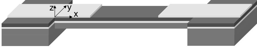
Figure 1.2: Structure of piezoelectric, micro-scale clamped-clamped resonator.
