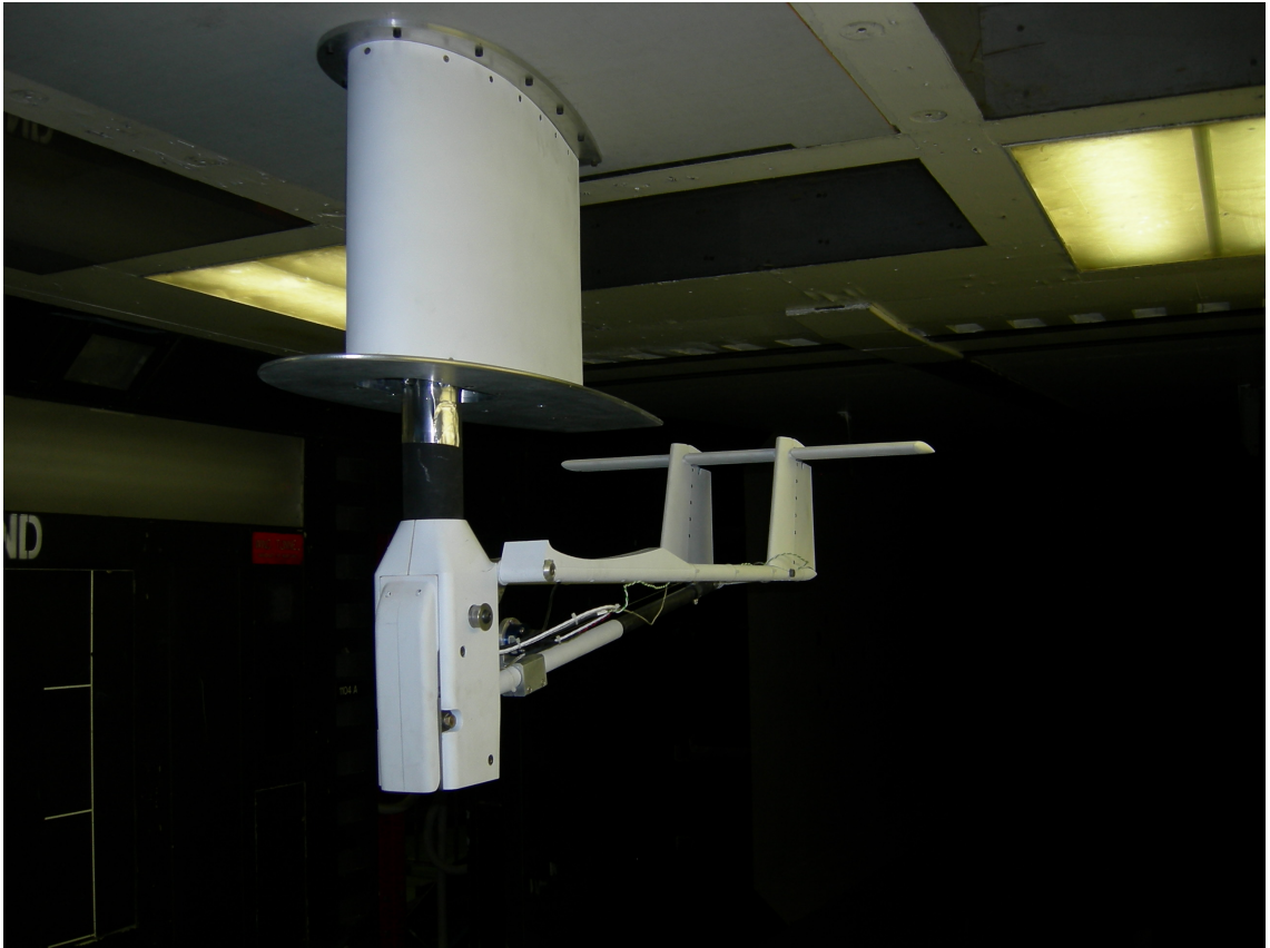
Figure 4.4: Photograph of the tail assembly of the PRM, with tail locked up in the fully deployed position.
