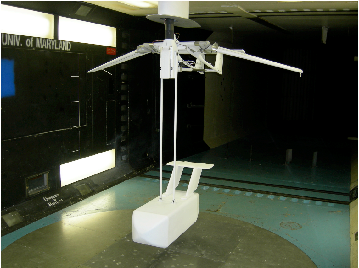
Figure 4.1: Photograph of the complete wind tunnel model in the Glenn L. Martin wind tunnel.
