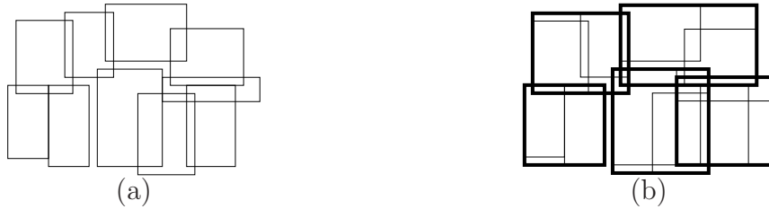
Figure 2.18: (a) A set of index data pages (b) are grouped to form slots, shown by thick-lined rectangles.
