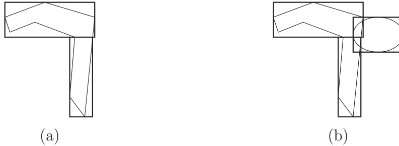
Figure 2.3: (a) In order to reduce dead space, an object can be approximated by two disjoint rectangles. (b) However, both rectangles might intersect a second object, thereby producing duplicate results.
