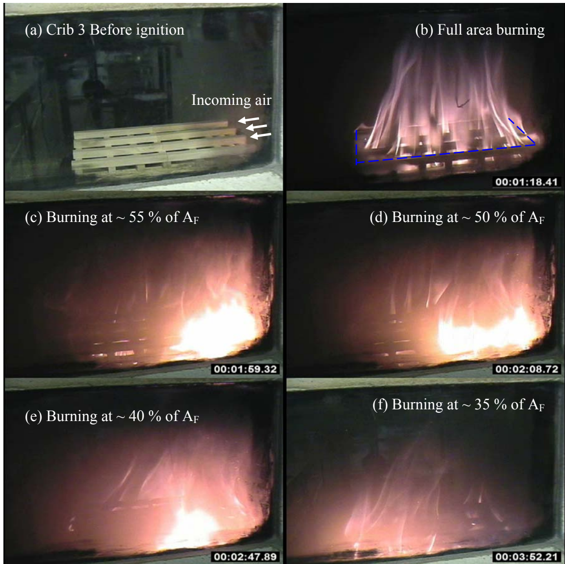
Figure 6.14 Caption showing estimation for the reduced burning area in under-ventilated burning, wood crib experiment Test C (Crib1W14x32)
