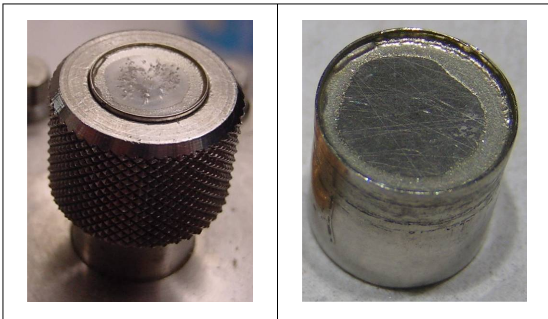
Figure 7.4: Dispenser Hermetic Seal (left); Ready for Vacuum Insertion (right)
