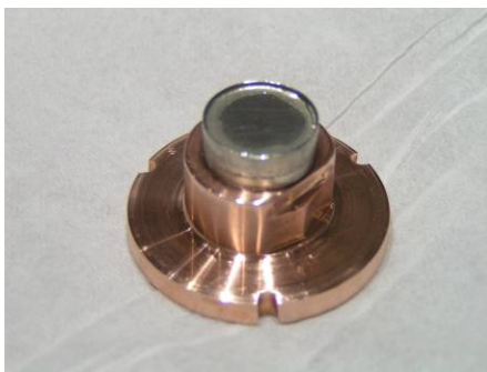
Figure 3.3: Dispenser Cathode with Heater Mount
