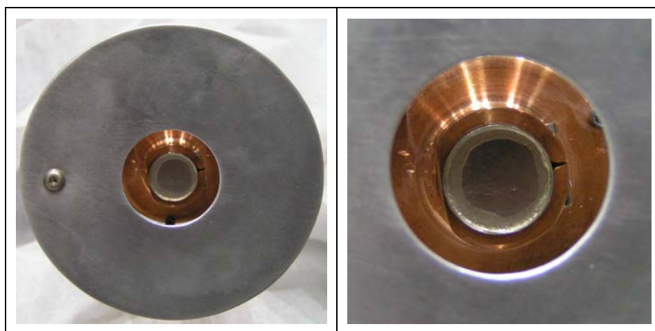
Figure 7.10: Front Face of Anode-Cathode Assembly Showing Mutual Alignment
