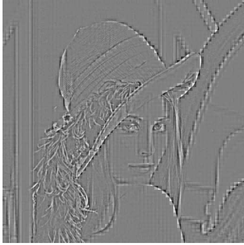
Figure 2.9: Approximated Lenna image by setting all DC coefficients to 0.
