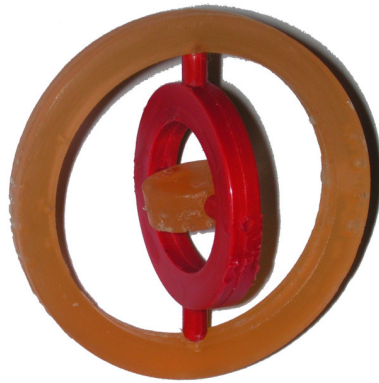
Figure 5.4. Multi-material molded gimbal mechanism [51].
