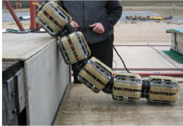
Figure 2.14. Omnitread robot climbing up a step [21].
