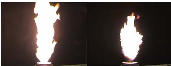
Figure 13. Images of forced 45°/50° flame. Left image: Flame near peak heat release. Right image: Flame near minimum heat release.
