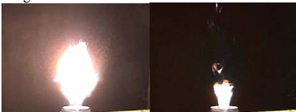
Figure 14. Images of 30°/50° co-swirling flame. Left image: Flame near peak heat release. Right image: Flame near minimum heat release.
