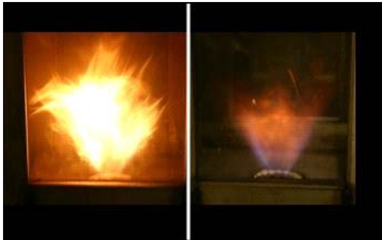
Figure B.3.2 Confined kerosene (left) and methanol (right) flames, at equal thermal load (from Linck, et al., August 2004)
