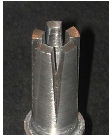
Figure 18. Detail of corrugated converging-diverging nozzle, showing corrugations and perforations through nozzle wall
