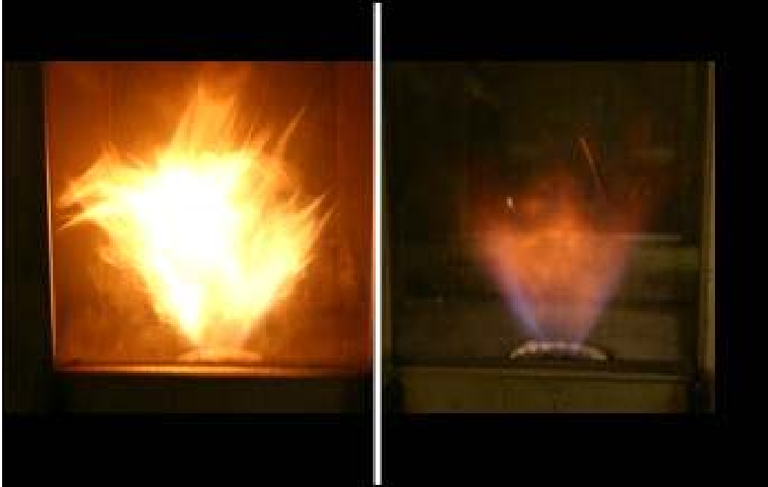
Figure 5. Confined flames using kerosene (left) and methanol (right) fuel.
