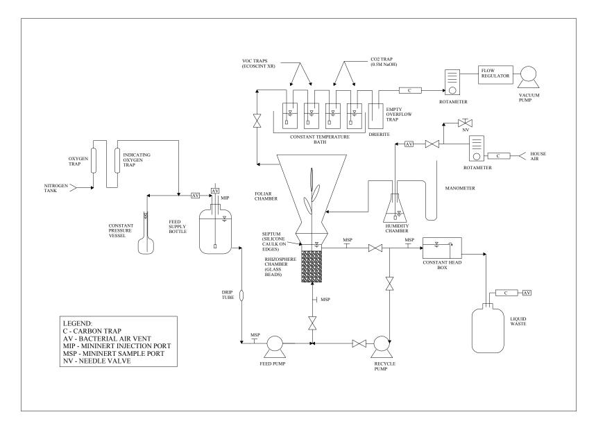
Figure 6-1: Overall design of the continuous-flow, completely-mixed bioreactor
