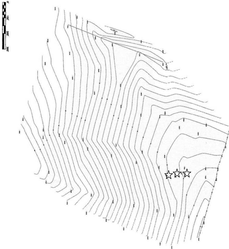
Figure C-2: Topographic map of Confined B watershed on Maryland dairy farm. Stars mark piezometer nests a, b, and c, moving from left to right on the flow line. Nests are 18 m apart. Bar is 300' long. Elevation changes 2' with each contour line.
