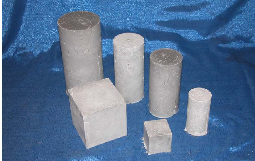
Figure 3.3.4-A: Compression cubes and cylinders including (clockwise from upper left) 4-in., 3-in. overlength, 3-in., and 2-in. diameter cylinders and 2 in. and 4 in. cubes
