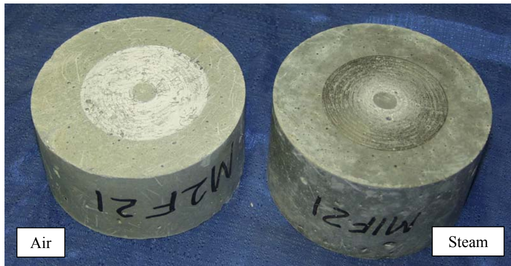
Figure 3.13.4-B: Steel cast surface Air and Steam Treated abrasion specimens after 8 and 10 minutes of abrading, respectively
