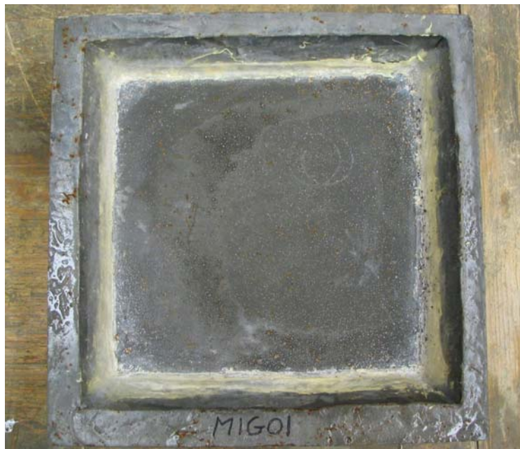
Figure 3.13.3-B: Scaling slab after ASTM C672 testing
