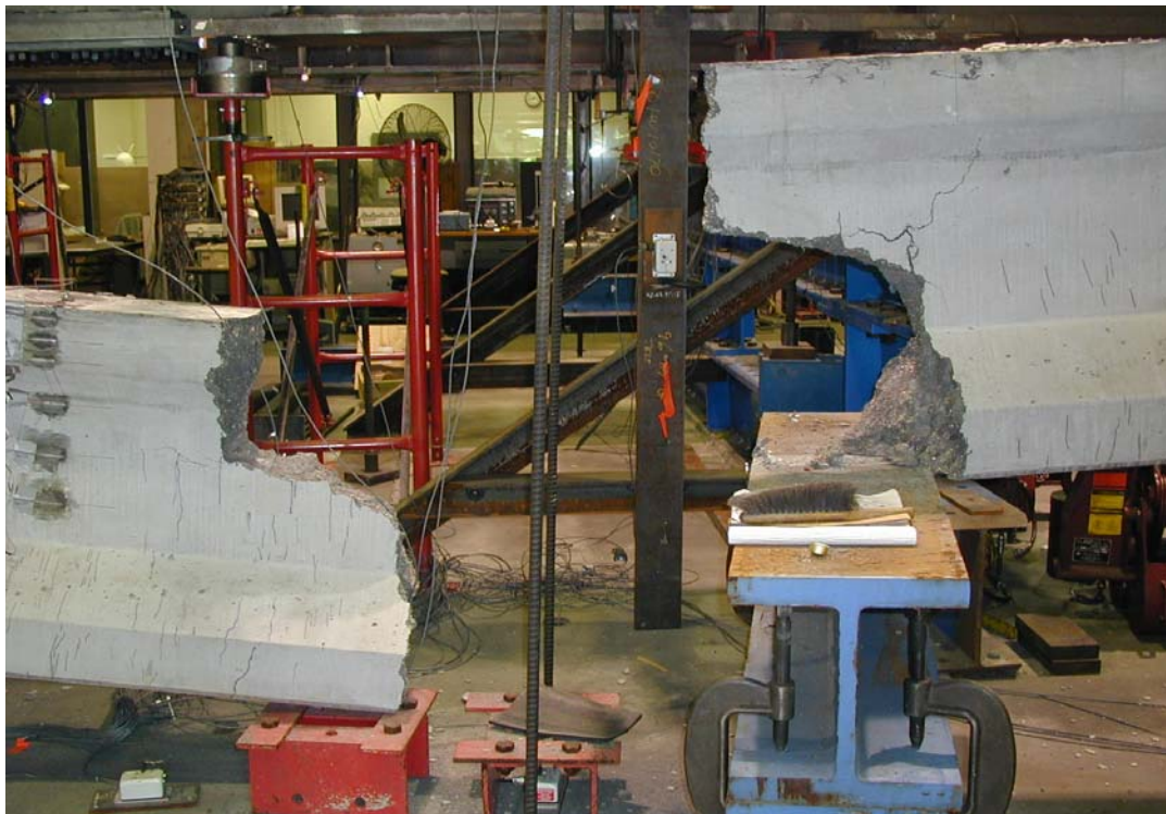
Figure 6.1-J: Girder 80F immediately after failure
