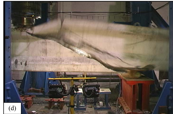
Figure 6.2.2-H: Failure of Girder 24S. (a) 1/15^{\text{th}} second before failure. (b) 1/30^{\text{th}} second before failure. (c) At failure. (d) 1/30^{\text{th}} second after failure.
