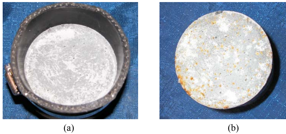
Figure 3.13.2-B: (a) Cylinder prior to and (b) after 90 days of chloride ponding
