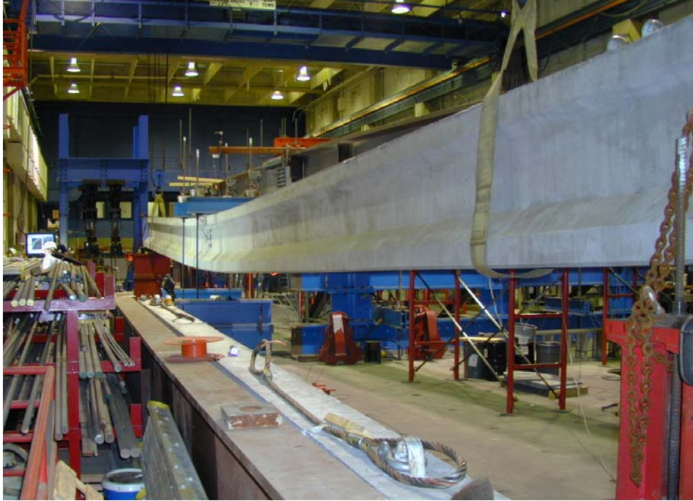
Figure 6.1-I: Girder 80F after approximately 17 in. of deflection
