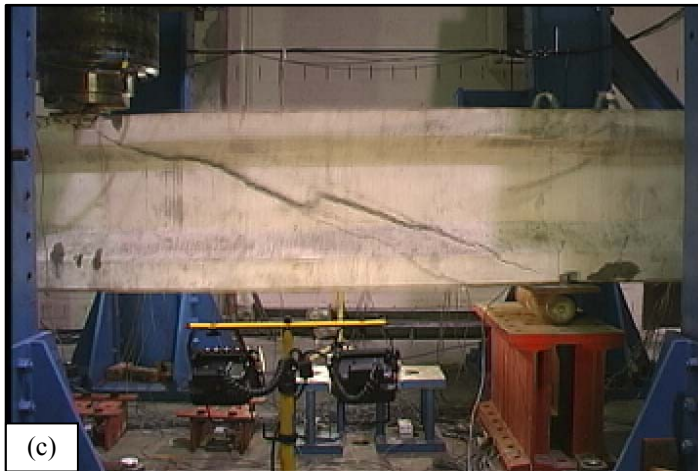
Figure 6.2.2-H: Failure of Girder 24S. (a) 1/15^{\text{th}} second before failure. (b) 1/30^{\text{th}} second before failure. (c) At failure. (d) 1/30^{\text{th}} second after failure.
