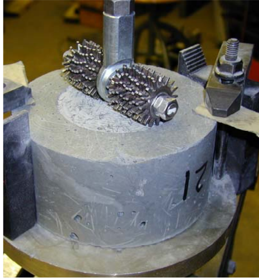
Figure 3.13.4-A: ASTM C944 abrasion test setup
