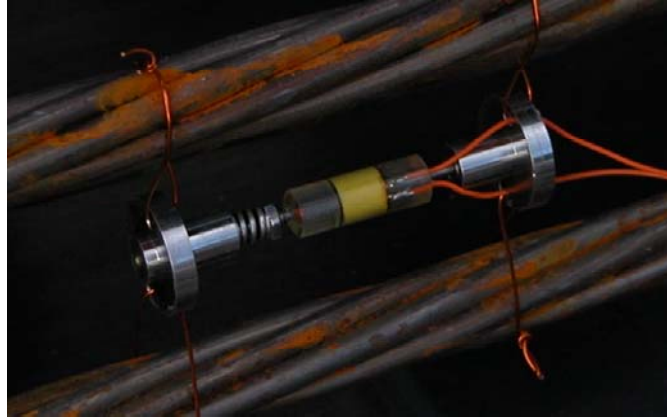
Figure 3.7.2-A: Embeddable vibrating wire gage
