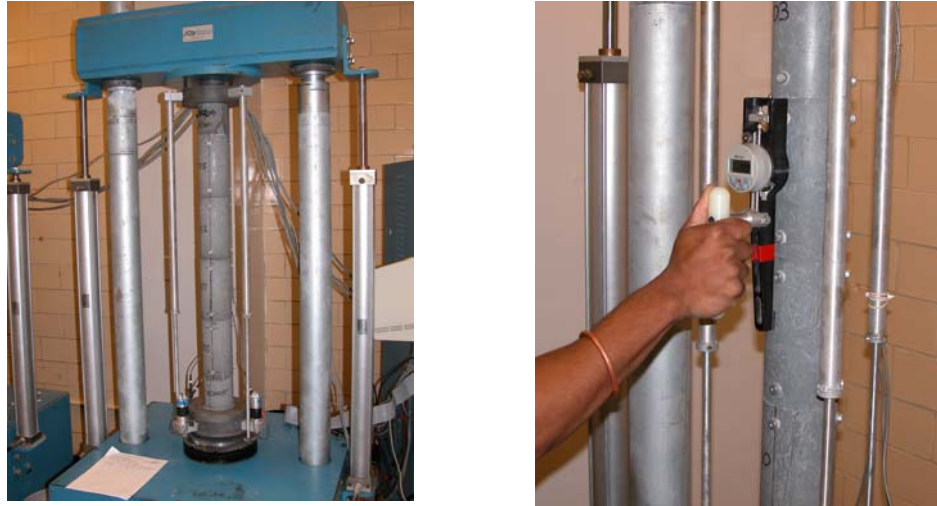
Figure 3.8.1-A: (a) Creep cylinders in load frame and (b) measurement of creep
