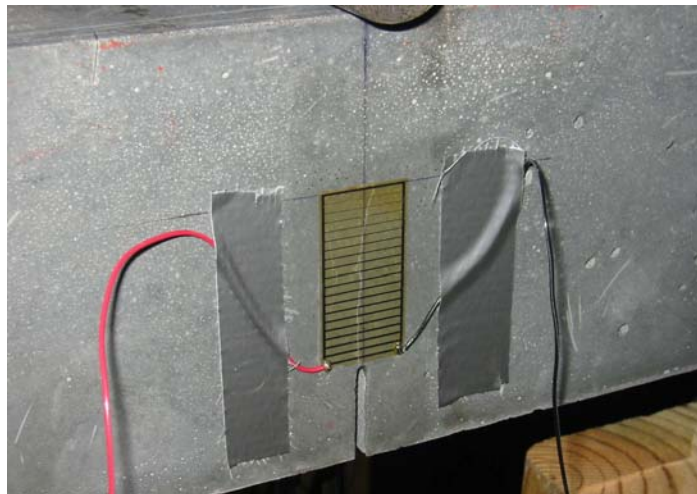
Figure 3.5-B: Resistance foil gage to monitor crack propagation
