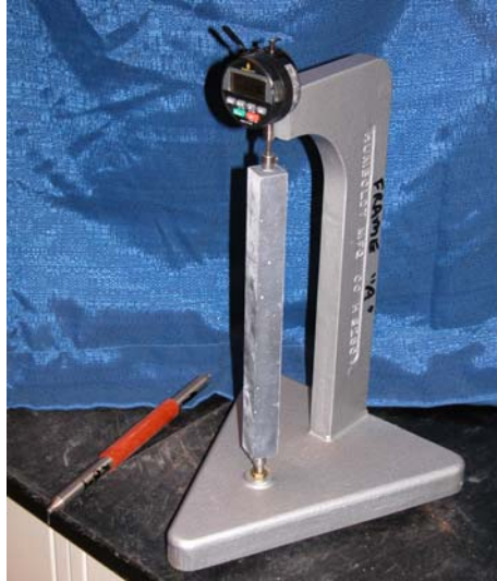
Figure 3.13.6-A: Length comparator for ASR measurements
