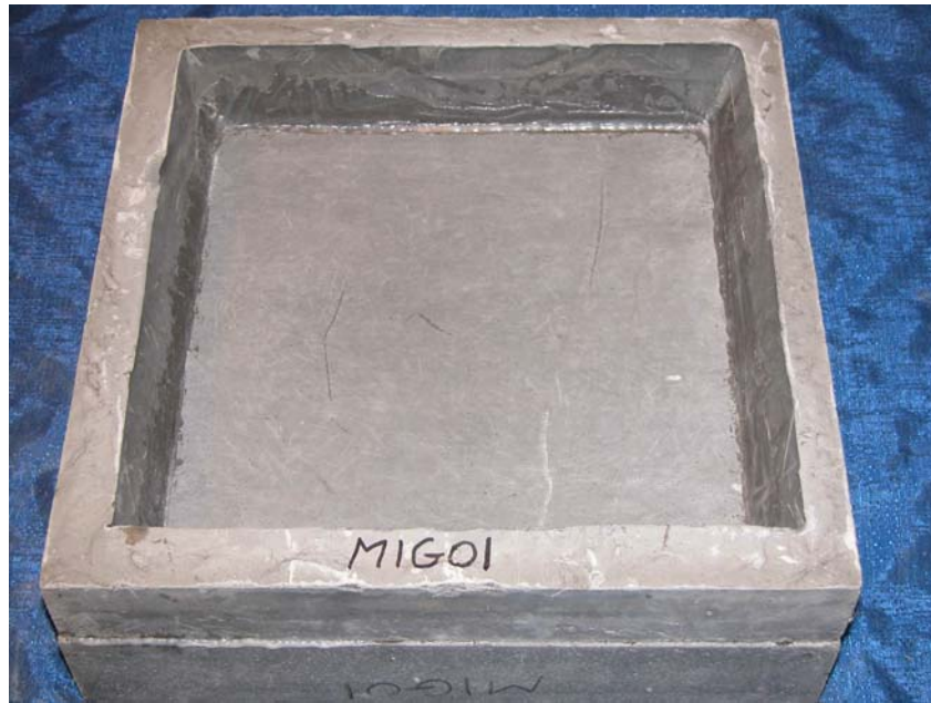
Figure 3.13.3-A: Scaling slab prior to the initiation of ASTM C672 testing
