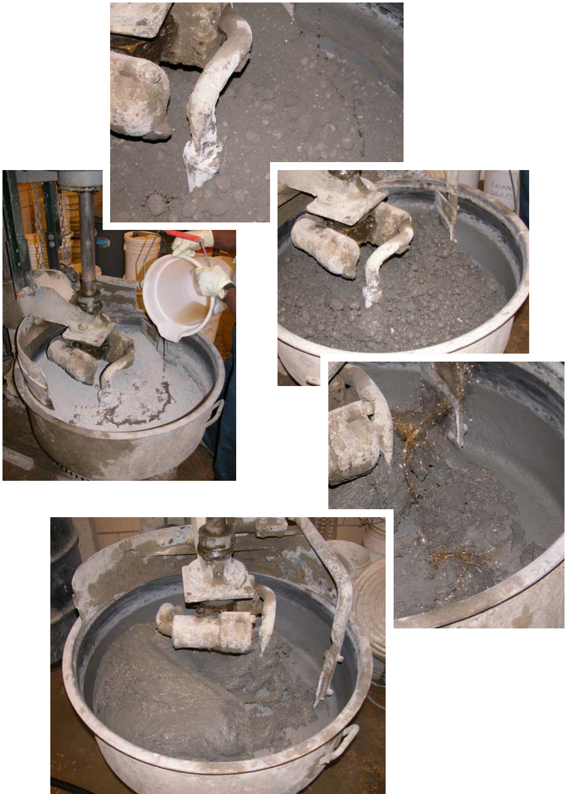
Figure 3.2-A: Mixing of UHPC including (clockwise from left) water addition, HRWA addition, pre-paste consistency, fiber addition, and finished mix
