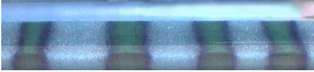
Figure 4.2: Picture of the “bands within bands” structures observed by Newey et al. [43]. The light blue particles are the largest, the dark blue particles are the intermediate sized ones and the green particles are the smallest.
