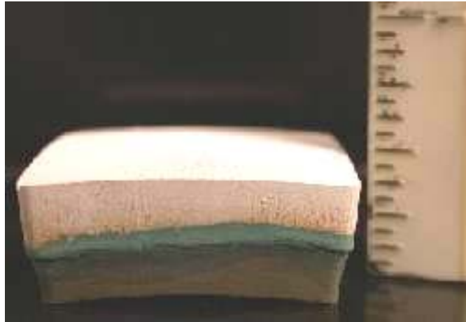
Figure 18. 12.7 mm FGM with 4 interlayers and bimodal alumina layer.
