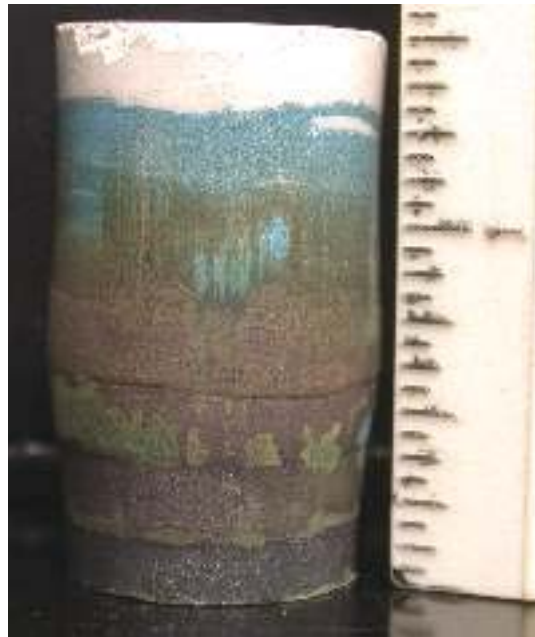
Figure 23. Crack-free circular specimen, roughly 38.1 mm, uniform layers.
