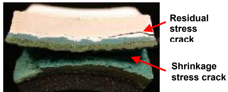
Figure 15. 12.7 mm FGM with 4 interlayers after sintering.
