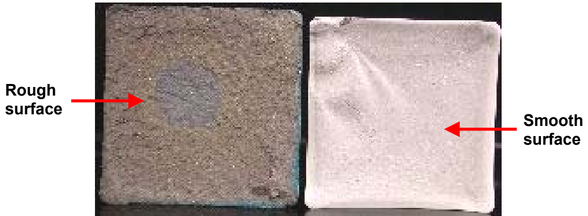
Figure 16. Fracture surfaces for shrinkage stress crack (left), and residual stress crack.
