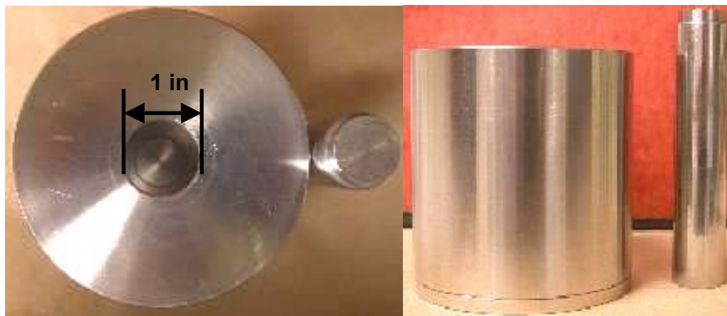
Figure 22. Die for circular specimens, with 1 in diameter.
