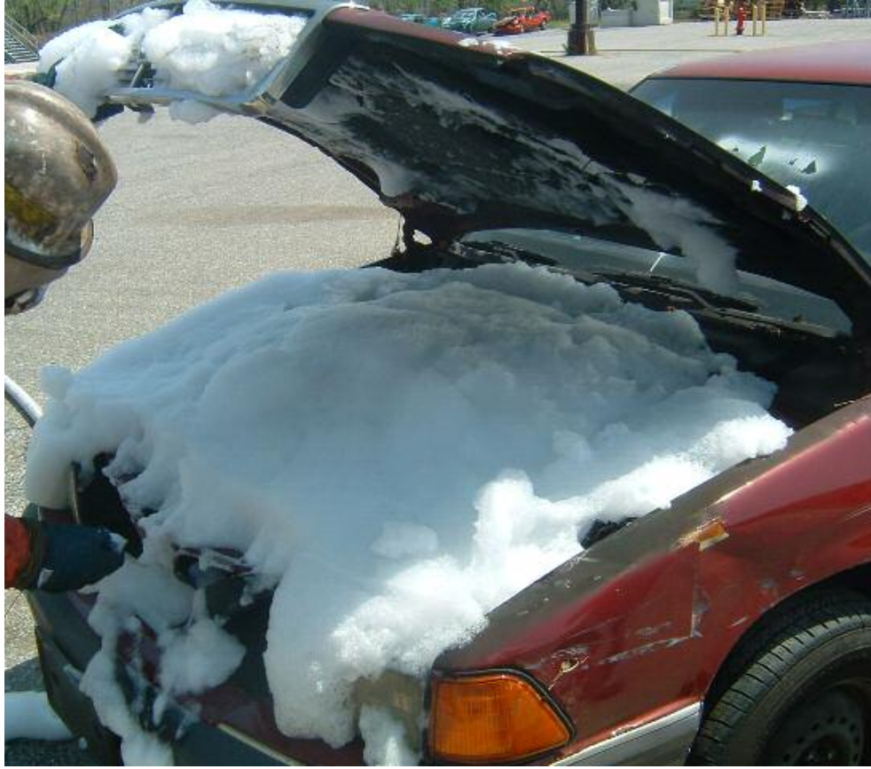
Figure 55: Foam Filled Chrysler Engine Compartment
