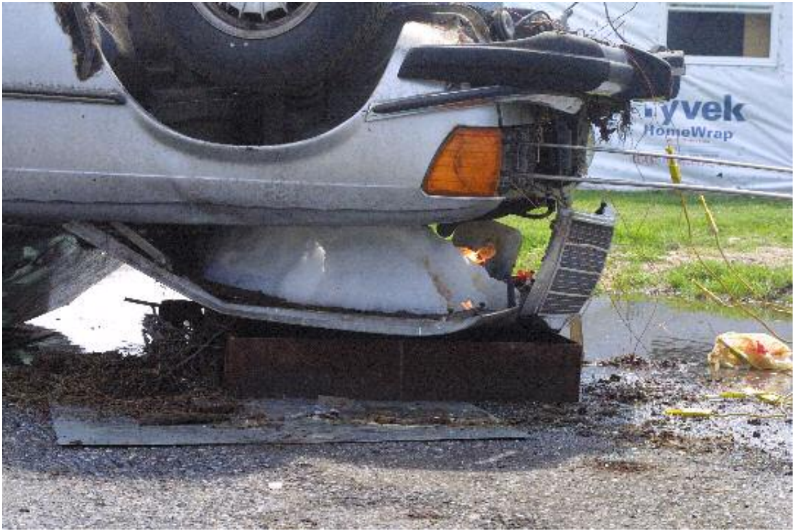
Figure 64: During Rollover Test, After Foam has Moved Over the Top of the Fire Pan.
