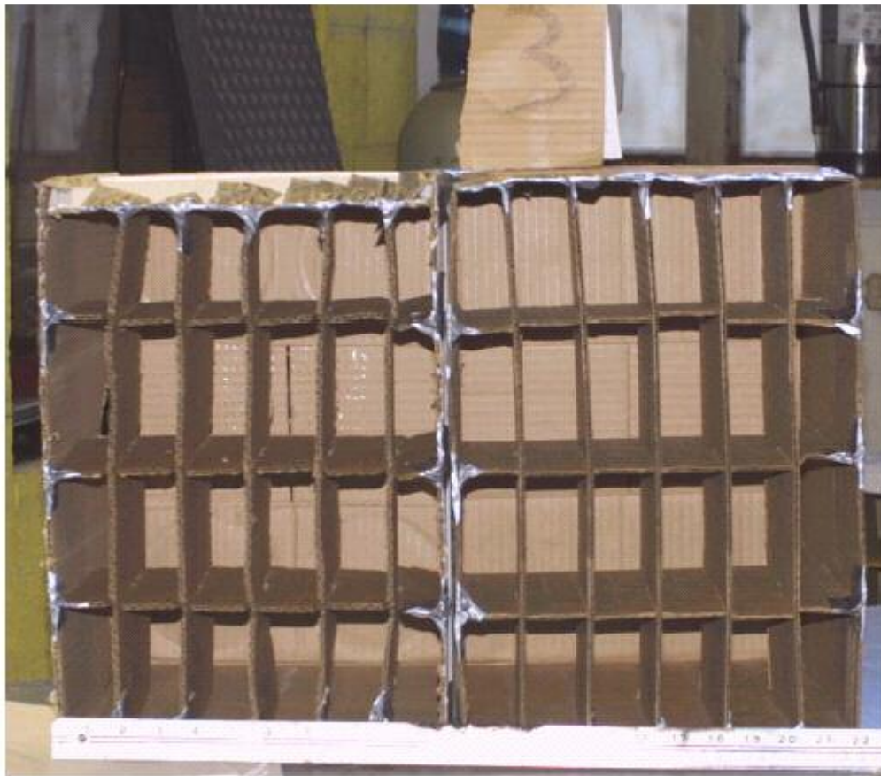
Figure 17: Box Set-Up #2: 8 cm 2 Channel Size
