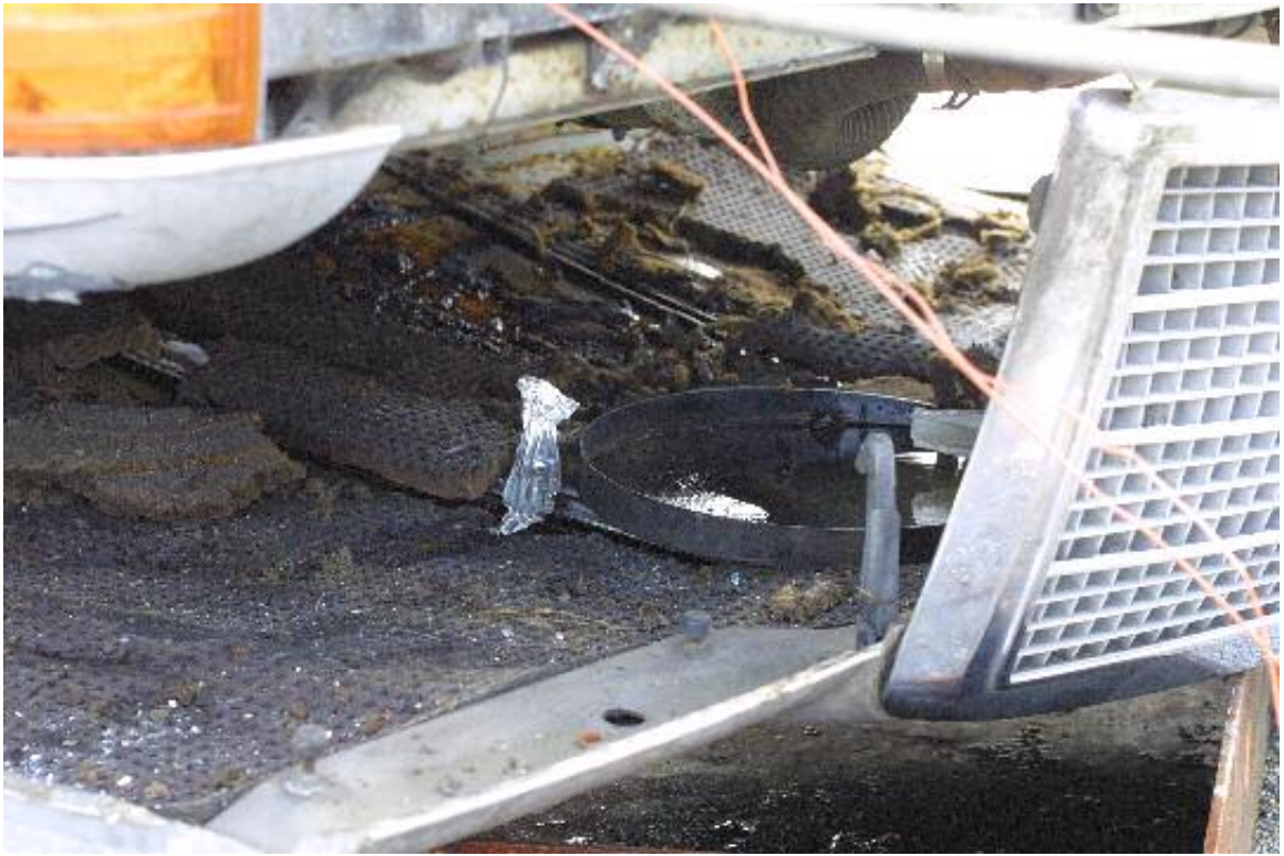
Figure 62: Position of Pan on Inside of Hood.
