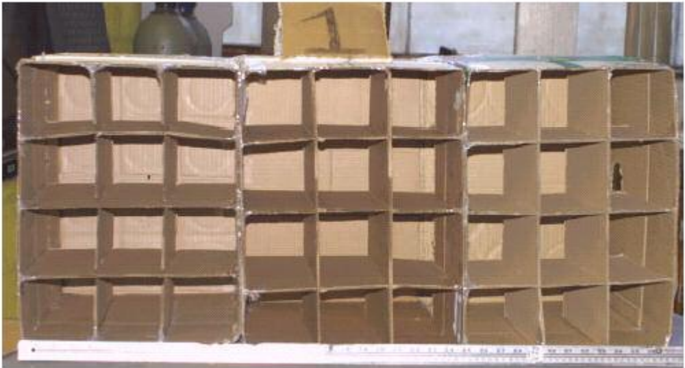
Figure 15: Inside View of Foam Flow Modeling Boxes Before Connected
