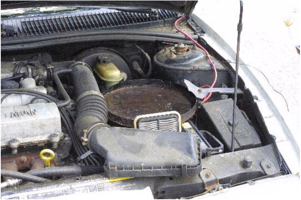
Figure 43: 0.3 m Diameter, Circular Pan, placed inside Saturn Engine Compartment
