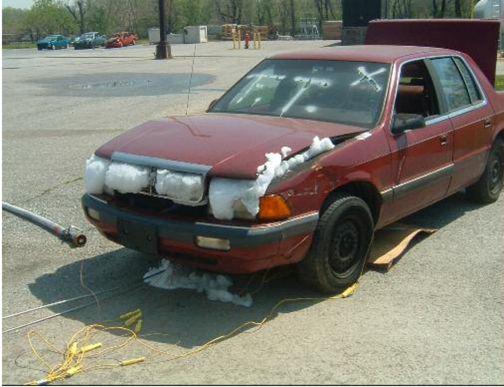
Figure 54: Foam Protruding from Chrysler at Completion of Test.
