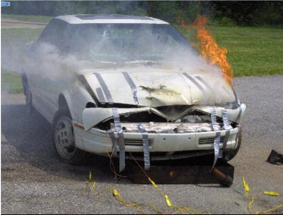
Figure 45: Saturn During Un-Suppressed Burn
