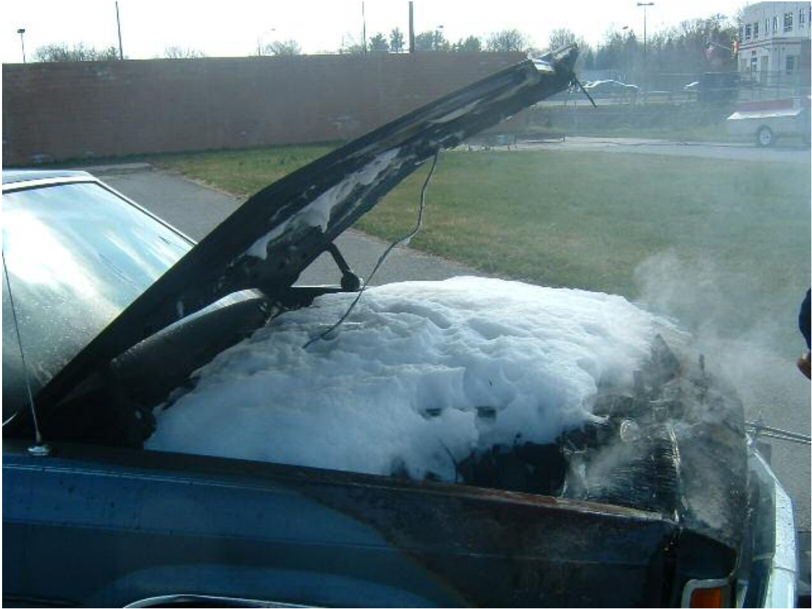
Figure 39: Foam Filled Engine Compartment Showing Area Around Pan Where Fire was Located and Foam Could Not Cover
