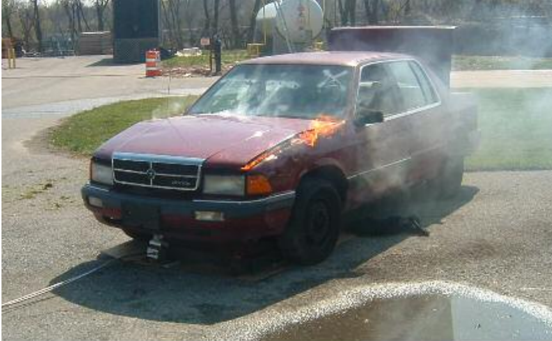
Figure 51: Chrysler During Test, Before Foam Has Reached the Fire
