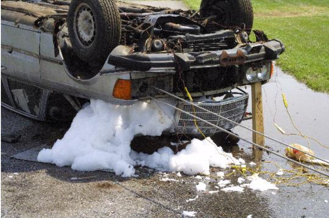
Figure 65: Movement of Foam from Sides of Hood.
