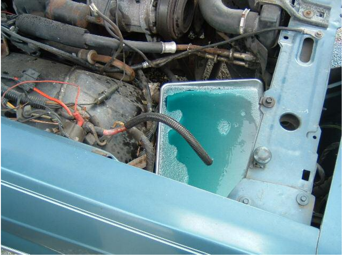
Figure 32: Aluminum Pan in Front Right of Ford LTD Engine Compartment and Filled with Gasoline
