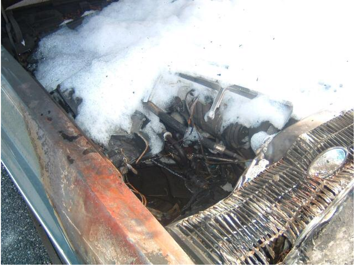
Figure 40: Close-Up View Showing Area Around Pan Where Fire was Located and Foam Could Not Cover
