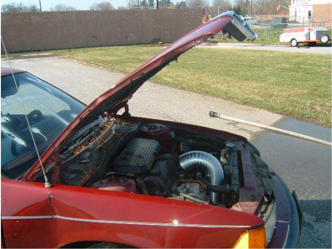
Figure 49: Position of HVAC Piping in Engine Compartment of Chrysler (Side View)
