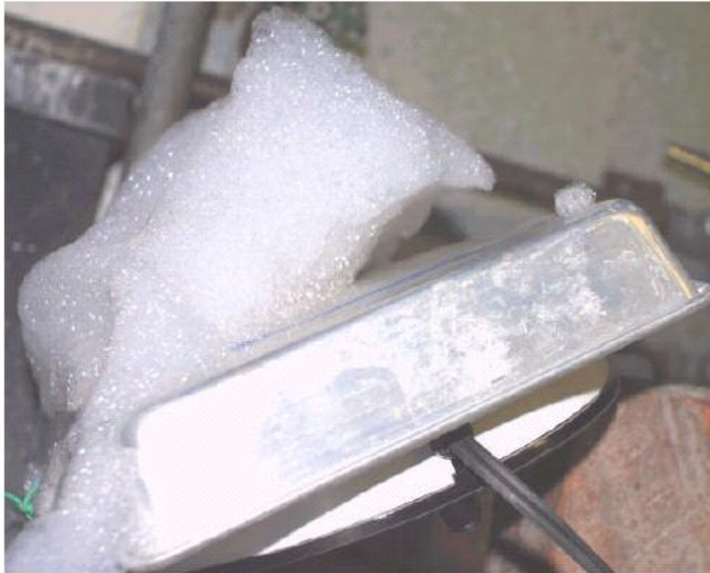
Figure 27: Hot Plate with Expansion Ratio = 220 Foam Showing Gap of 30 mm
