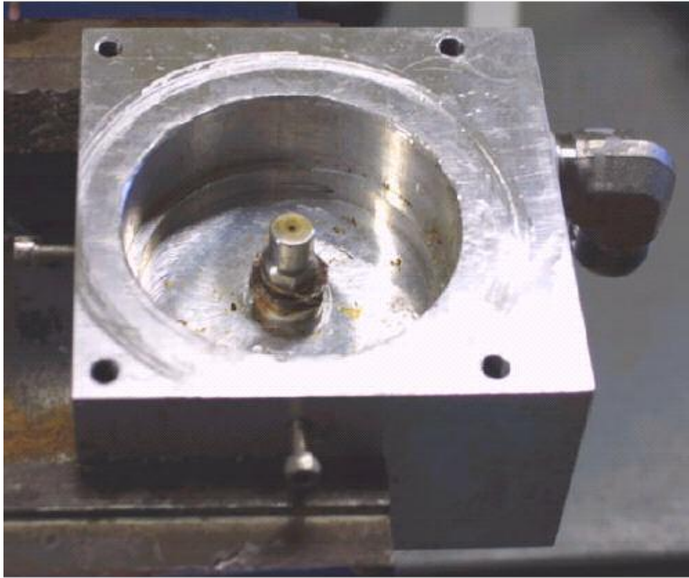
Figure 8: Foam Generator (top view) and Liquid Spray Nozzle
