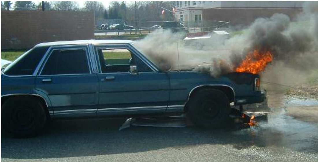
Figure 38: Burn #2 on Ford LTD: Immediately Prior to Fire Being Extinguished.
