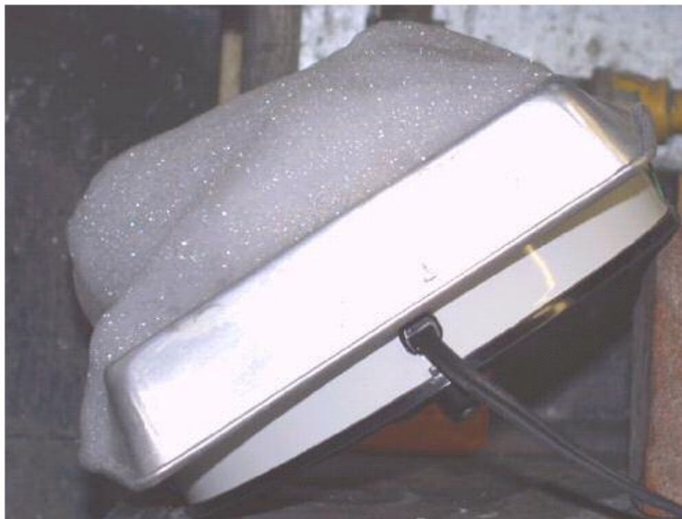
Figure 26: Hot Plate with Foam Applied: Expansion Ratio = 220
