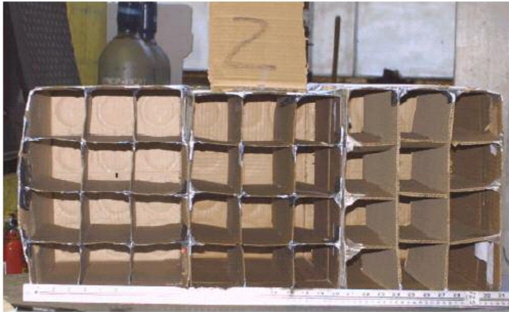
Figure 17: Box Set-Up #2: 8 cm 2 Channel Size
