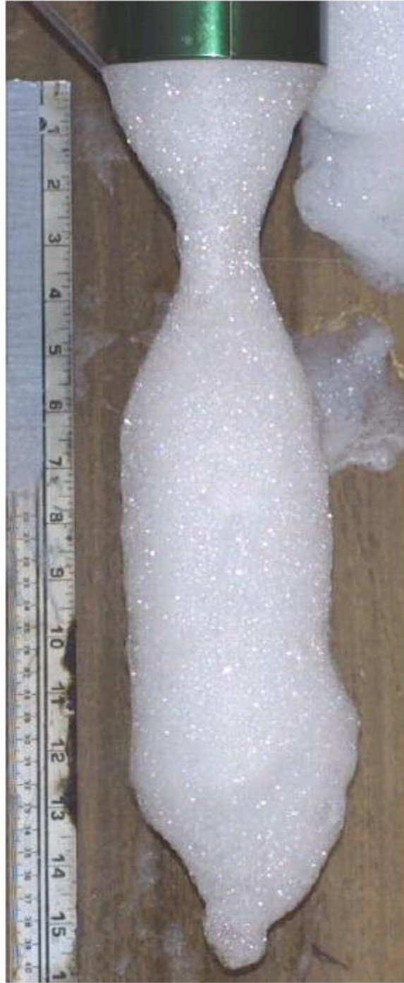
Figure 23: Foam Hang Test: Expansion Ratio = 220, Diameter of Pipe = 0.1 m
