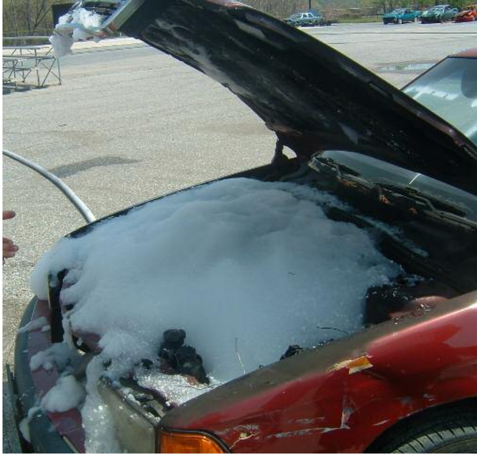
Figure 56: Foam Filled Chrysler Engine Compartment After 10 Minutes
