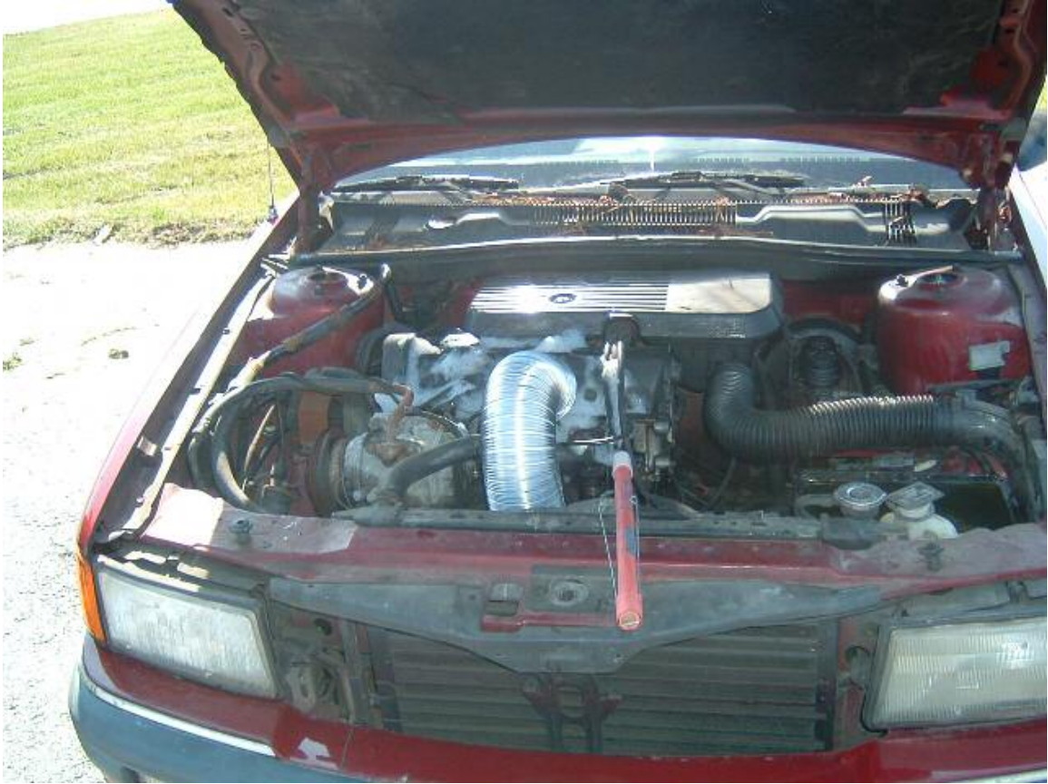
Figure 50: Position of HVAC Piping in Engine Compartment of Chrysler (Front View)
