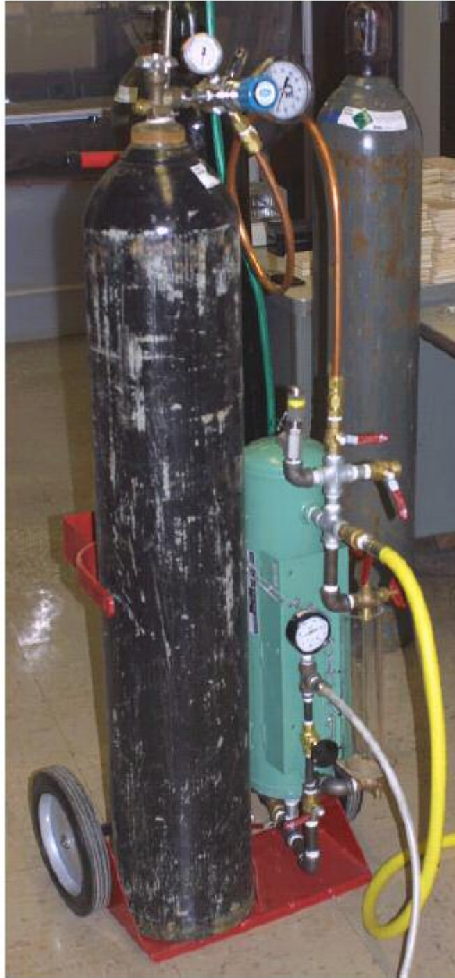
Figure 1: Foam Generating System
