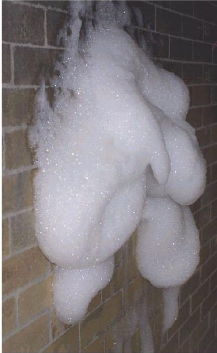
Figure 24: Foam Hanging From Wall: Expansion Ratio = 220
