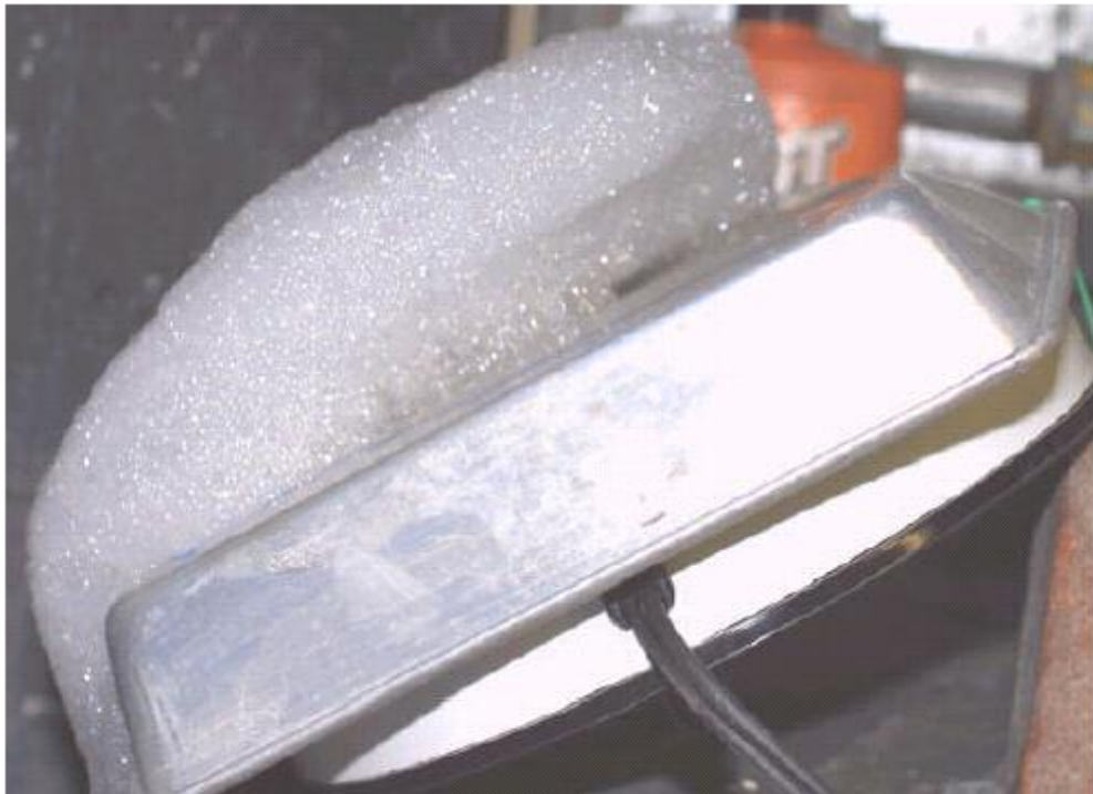
Figure 28: Hot Plate with Expansion Ratio = 220 Foam Showing Gap of 30 mm
