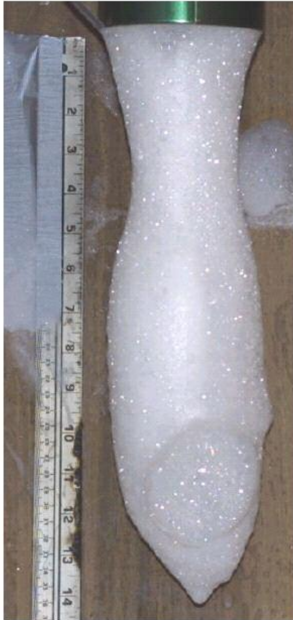
Figure 22: Foam Hang Test: Expansion Ratio = 220, Diameter of Pipe = 0.1 m
