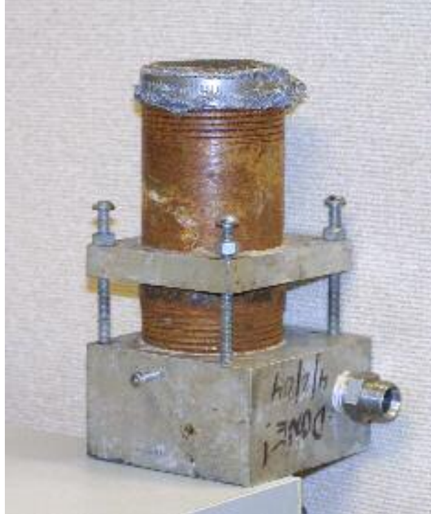
Figure 33: Foam Nozzle with Clamping Device Added to Prevent Gas Leakage
