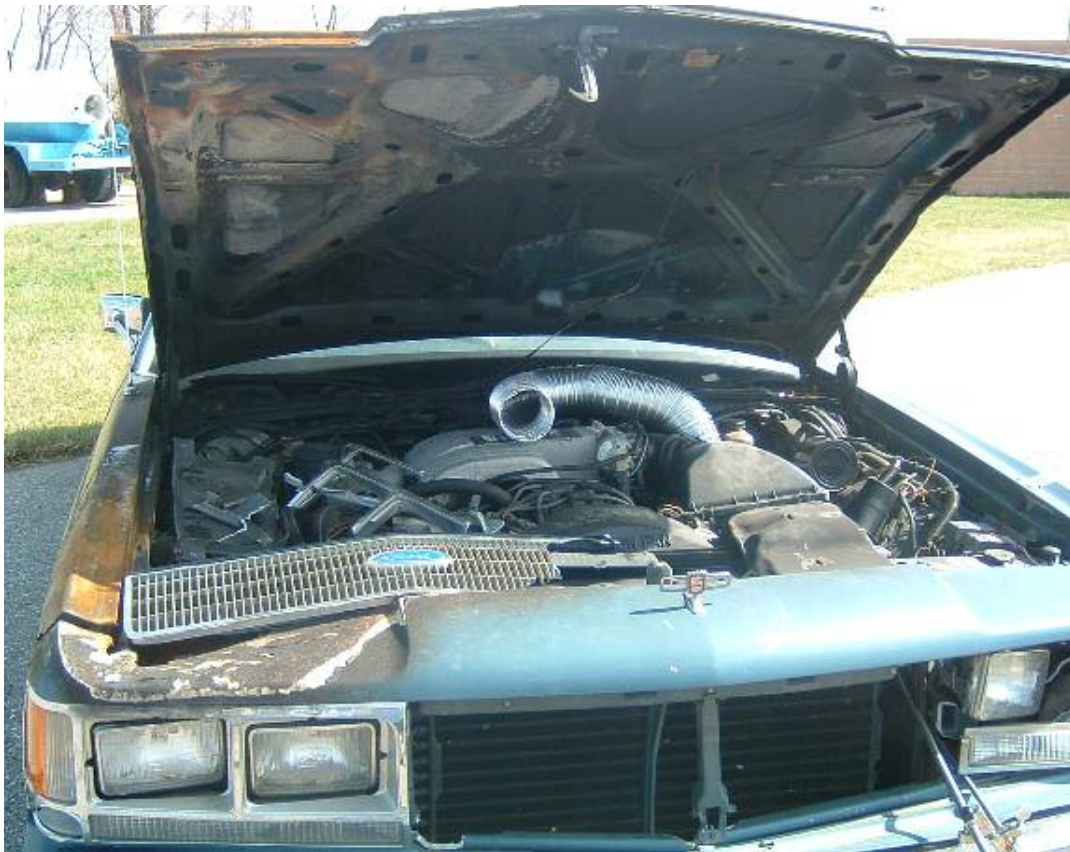
Figure 31: Insertion Point of Stainless Steel Tubing into Ford LTD Engine Compartment through Grill, Position of Foam Generator and Position of HVAC Piping
