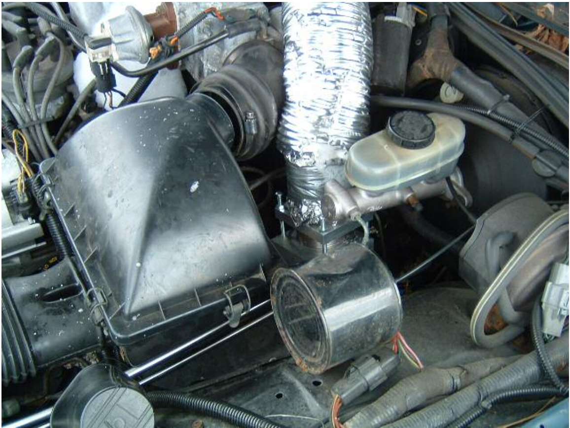
Figure 30: Position of Foam Generator Nozzle within Engine Compartment
