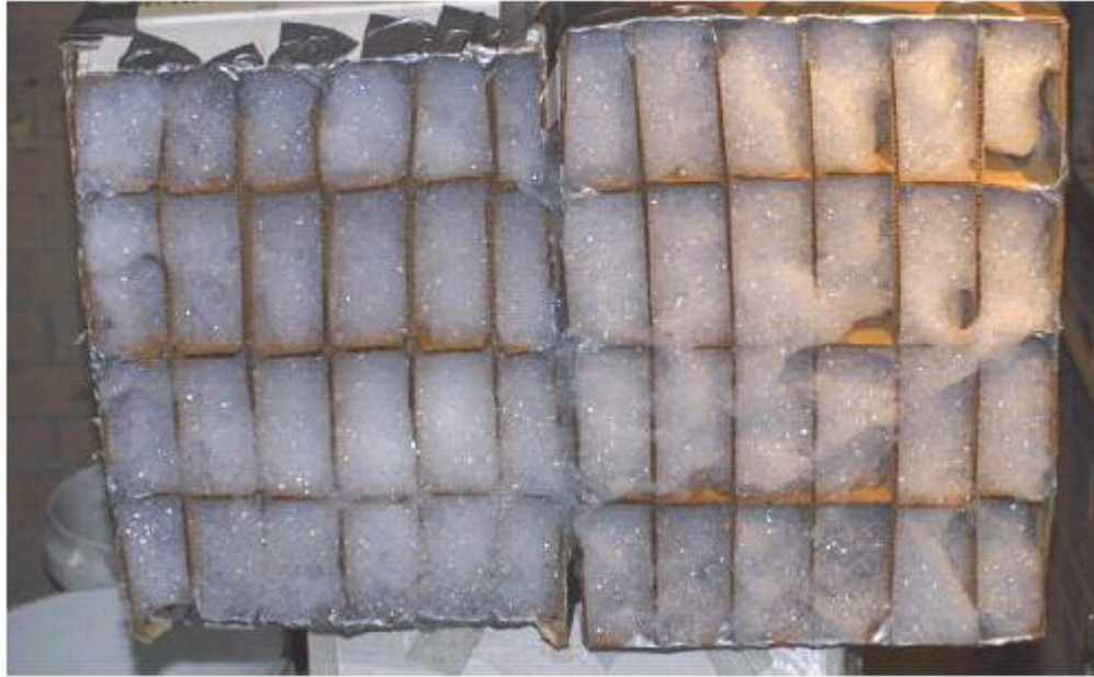
Figure 21: Box Set-Up #3 w/ 200 Expansion Ratio Foam
