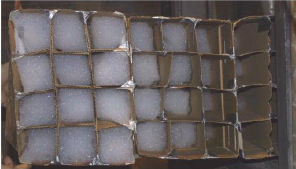
Figure 19: Box Set-Up #1 w/ 120 Expansion Ratio Foam
