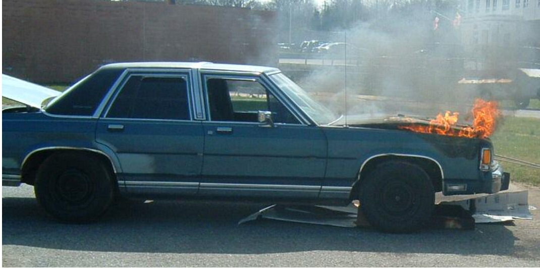
Figure 37: Burn #2 on Ford LTD: Early in Test.
