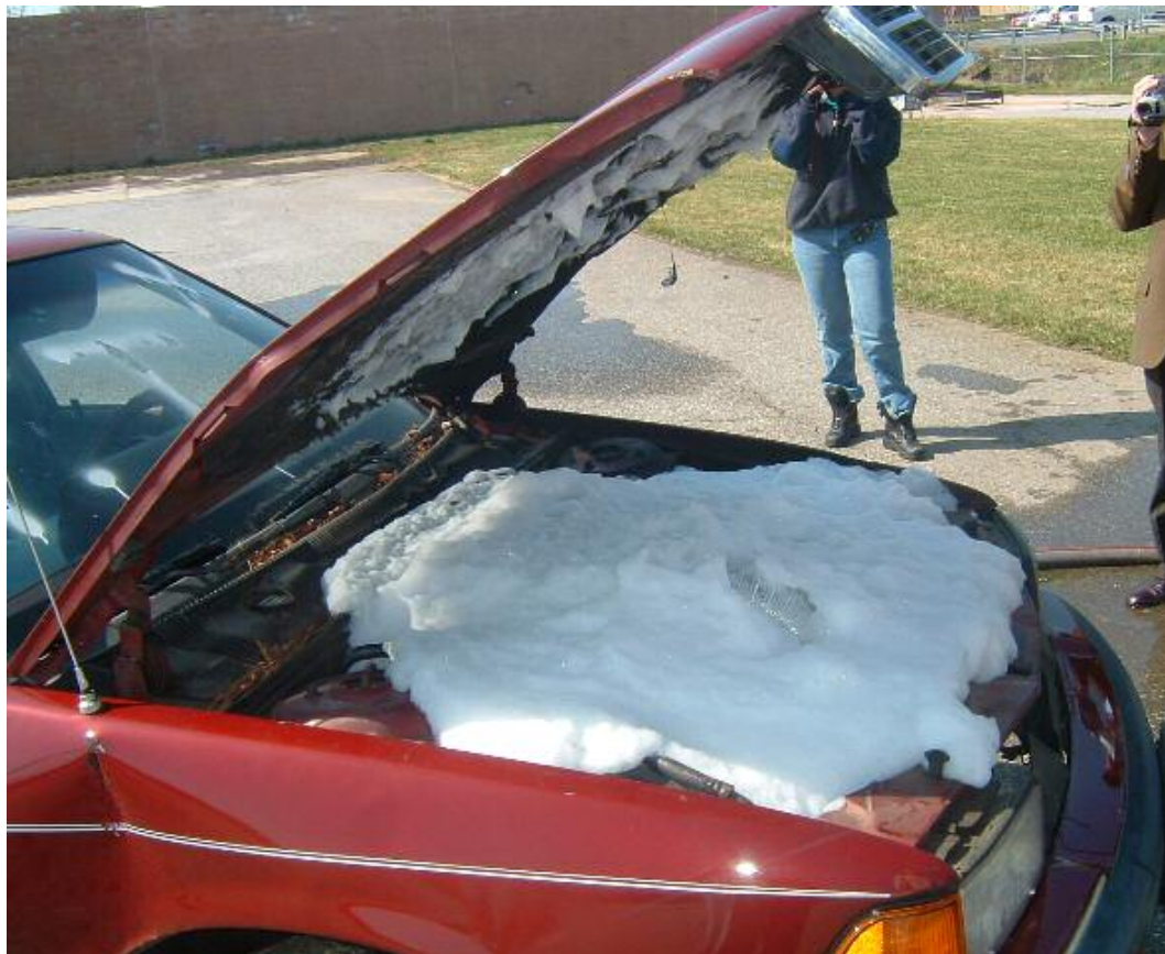
Figure 52: Foam Filled Engine Compartment of Chrysler (Side View)
