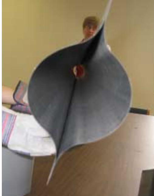
Figure 4-21: Boom cross-section profile after prolonged stowage
