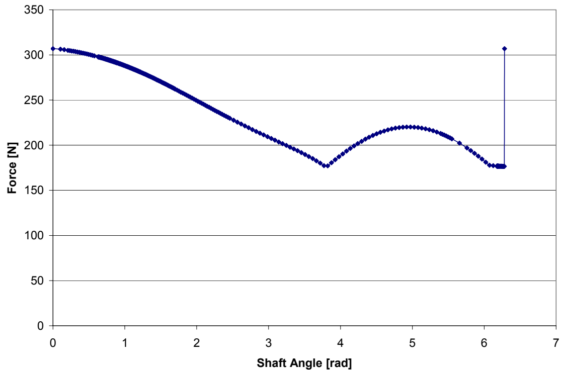
Figure 16: Rolling Piston/Vane Contact Force versus Shaft Angle
